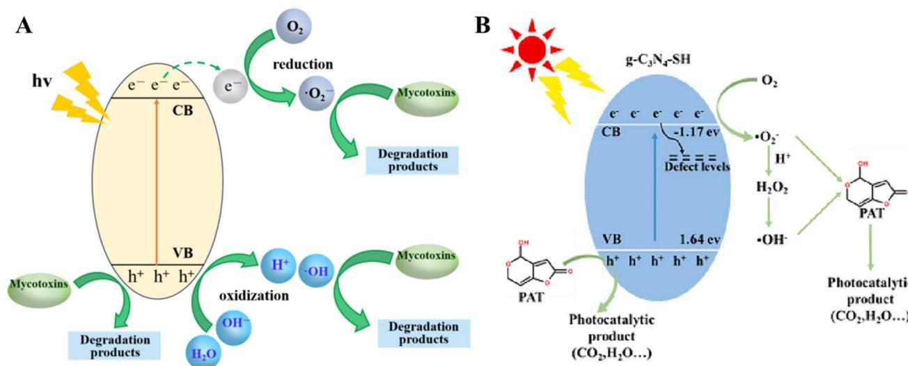
Fig. 4 Schematic of a typical photocatalytic mechanism. (A) Schematic representation of a typical photocatalytic mechanism;<sup>68</sup> (B) schematic representation of the photocatalytic mechanism of KG-5 photocatalyst.
