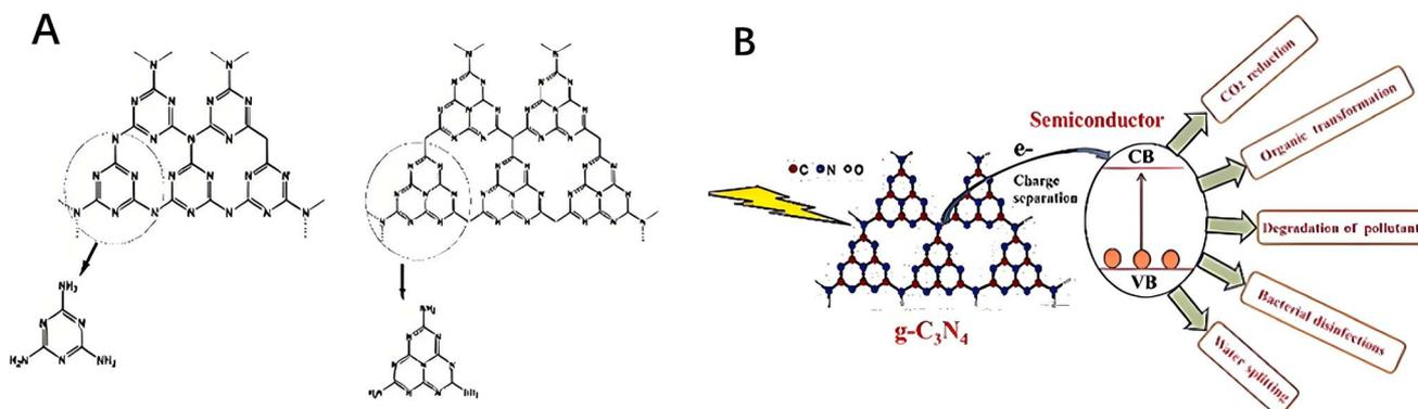
Fig. 2 Photocatalytic reactions of carbon–nitride-based materials. (A)  $g\text{-C}_3\text{N}_4$  has two structures, namely the triazine (a) and the tri-*s*-triazine.<sup>17</sup> (B) Mechanism and application of  $g\text{-C}_3\text{N}_4$  photocatalytic reaction.<sup>18</sup>
