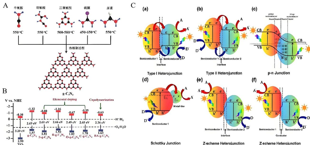
Fig. 5 Energy band structure of doped g-C<sub>3</sub>N<sub>4</sub> synthesized by thermal polycondensation. (A) g-C<sub>3</sub>N<sub>4</sub> was synthesized from several precursors by thermal polycondensations.<sup>80</sup> (B) Energy band diagrams of TiO<sub>2</sub> and g-C<sub>3</sub>N<sub>4</sub>, along with their commonly used dopant species.<sup>80</sup> (C) Illustrative representation of the energy band configuration of various types of heterojunctions.<sup>81</sup>
