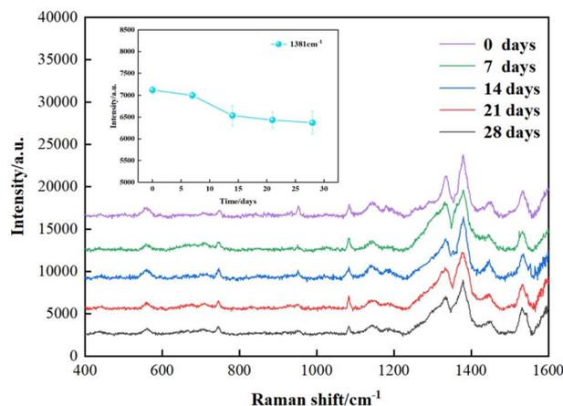
Fig. 8 SERS spectra of  $10^{-4}\text{ M}$  thiram using  $\text{Fe}_3\text{O}_4/\text{GO}/\text{Ag}$  as substrate that has been stored for various periods.
