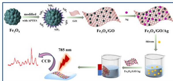
Scheme 1 Illustration of the fabrication process of Fe<sub>3</sub>O<sub>4</sub>/GO/Ag with its application in SERS.
