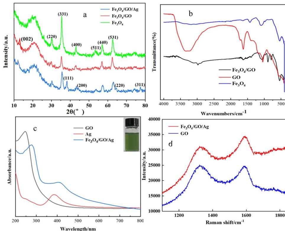
Fig. 1 (a) XRD patterns of  $\text{Fe}_3\text{O}_4$ , GO, and  $\text{Fe}_3\text{O}_4/\text{GO}/\text{Ag}$ ; (b) IR of  $\text{Fe}_3\text{O}_4$ , GO, and  $\text{Fe}_3\text{O}_4/\text{GO}/\text{Ag}$ ; (c) ultraviolet-visible absorption spectra of each sample (insert: silver nanosol); and (d) Raman spectra of GO in blue line and Raman spectra of  $\text{Fe}_3\text{O}_4/\text{GO}/\text{Ag}$  in red line.
