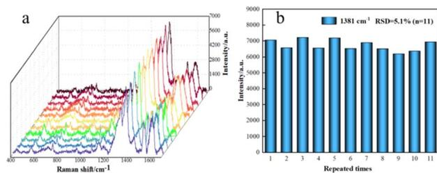
Fig. 10 (a) SERS spectra of 10<sup>-4</sup> M thiram from 11 randomly selected Fe<sub>3</sub>O<sub>4</sub>/GO/Ag composite microspheres. (b) Raman intensity distribution of 1381 cm<sup>-1</sup> peak from the 11 spectra.
