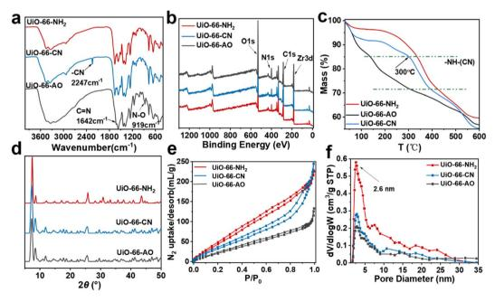
Fig. 3 Characterization of UiO-66-NH<sub>2</sub> before and after modification. (a) FT-IR spectra, (b) XPS spectra, (c) TG curves, (d) PXRD patterns, (e)  $N_2$  adsorption/desorption isotherms, and (f) pore size distributions of UiO-66-NH<sub>2</sub>, UiO-66-CN, and UiO-66-AO.
