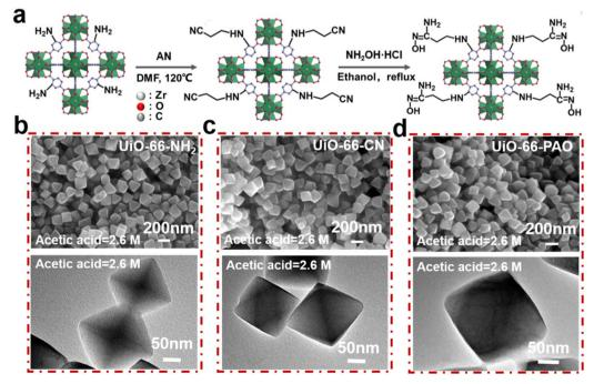
Fig. 2 (a) UiO-66-AO synthesis process. SEM and TEM images of (b) UiO-66-NH<sub>2</sub>, (c) UiO-66-CN, and (d) UiO-66-AO.
