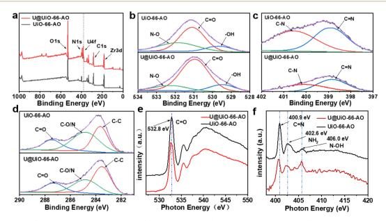
Fig. 6 (a) XPS spectra, (b) O 1s spectra, (c) N 1s spectra, (d) C 1s spectra and (e) O k-edge of NEXAFS and (f) N k-edge of NEXAFS of UiO-66-AO and U@UiO-66-AO.
