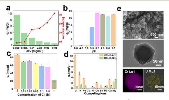
Fig. 4 (a) Effect of the mass-to-volume ratio on adsorption performance. (b) Influence of pH on  $UO_2^{2+}$  adsorption ( $c_0 = 500$  ppb, t = 24 h), (c) the effect of anion  $Cl^-$  concentration on  $UO_2^{2+}$  adsorption ( $c_0 = 2.0$  ppm, t = 24 h). (d) Adsorption in simulated seawater (ion concentrations provided in Table S1,† t = 24 h). (e) SEM and TEM of UiO-66-AO after the adsorption of  $UO_2^{2+}$  in seawater, and its Zr, and U elemental mapping photographs.
