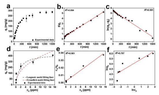
Fig. 5 (a) Impact of contact time on  $UO_2^{2+}$  adsorption ( $c_0 = 8$  ppm, t = 24 h), (b) the pseudo-second-order and (c) the pseudo-first-order kinetic model linearized plots for  $UO_2^{2+}$  adsorption, (d) impact of  $UO_2^{2+}$  concentration on the adsorption ( $c_0 = 0.1-20.0$  ppm, t = 24 h), (e and f) fitting results for the Langmuir and Freundlich isothermal adsorption models of UiO-66-AO.
