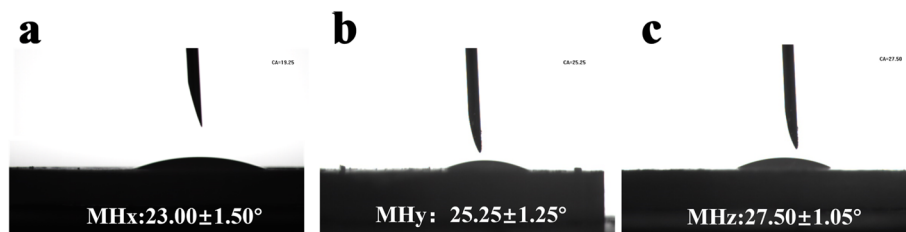
Fig. 5 WCA images of MHx (a), MHy (b), and MHz (c).
