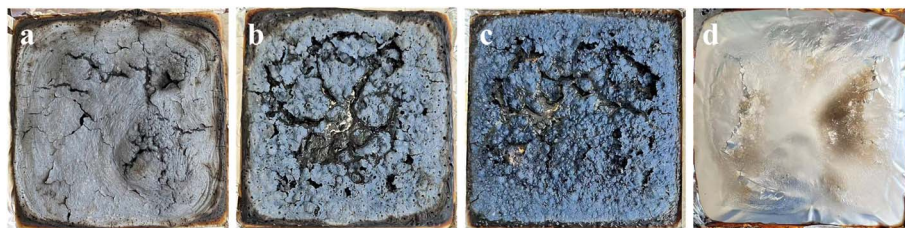
Fig. 10 Digital images of the char residues of EVA/MHx60 (a), EVA/MHy60 (b), EVA/MHz60 (c), and pure EVA (d).
