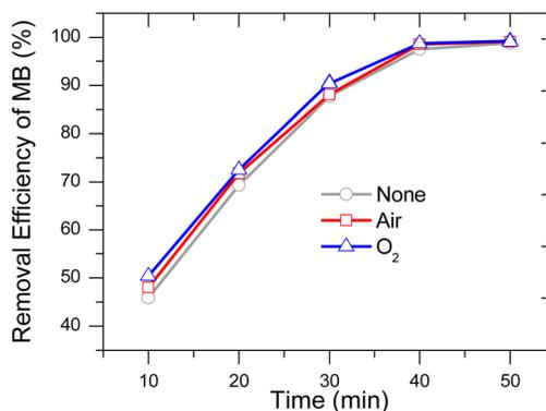
Fig. 7 Effect of air/O<sub>2</sub> aeration into the MB solution on the MB removal efficiency ( $d = 10$  mm; initial MB concentration =  $10$  mg  $\text{L}^{-1}$ ; stirring speed =  $150$  rpm; flow rate of air/O<sub>2</sub> =  $1.6$  L  $\text{min}^{-1}$ ).
