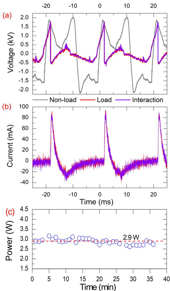
Fig. 2 Typical voltage and current of the plasma jet: (a) voltage waveforms, (b) current discharge, and (c) discharge power (Ar flow rate = 3.5 L min<sup>-1</sup>).
