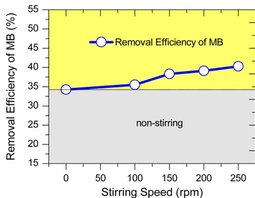
Fig. 4 Effect of stirring solution on the MB removal efficiency ( $d = 10$  mm; initial MB concentration = 10 mg L<sup>-1</sup>; interaction time = 10 min).
