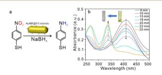
Fig. 5 (a) Reaction scheme for the conversion of 4-NTP to 4-ATP in the presence of NaBH4 and AuNR@Pd islands; (b) UV-vis of 4-NTP reduction catalyzed by AuNR@Pd islands.
