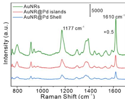
Fig. 4 SERS spectra of CV acquired from different substrates.
