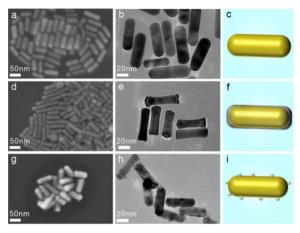
Fig. 2 SEM, TEM images and schematic diagram of (a-c) AuNRs; (d-f) AuNR@Pd shell; and (g-i) AuNR@Pd islands.
