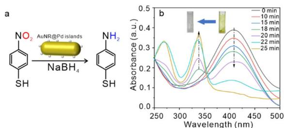
Fig. 5 (a) Reaction scheme for the conversion of 4-NTP to 4-ATP in the presence of NaBH<sub>4</sub> and AuNR@Pd islands; (b) UV-vis of 4-NTP reduction catalyzed by AuNR@Pd islands.
