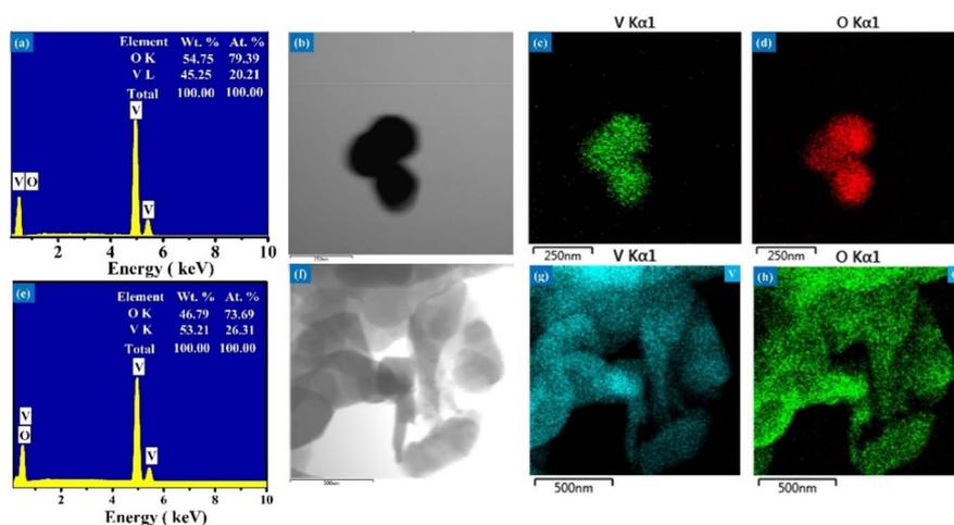
Fig. 2 Elemental composition and distribution of  $V_2O_5$  nanosheets and microflowers (a) and (e) EDS spectra showing the elemental composition of  $V_2O_5$  nanosheets and microflowers, respectively. (b)–(d), (f)–(h) Elemental mapping images displaying the uniform distribution of vanadium (V) and oxygen (O) in the  $V_2O_5$  nanosheets (b)–(d) and microflowers (f)–(h).
