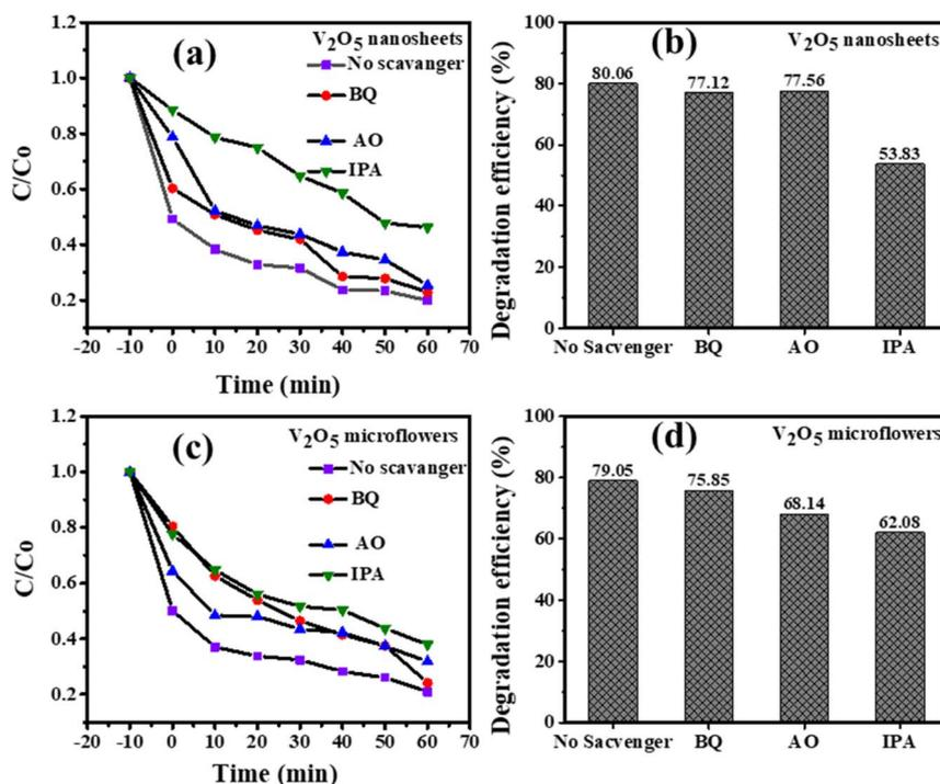
Fig. 11 The effect of radical scavengers on the photodegradation of MB by (a) and (b)  $V_2O_5$  nanosheets and (c) and (d) microflowers photocatalysts after 60 minutes of light irradiation.
