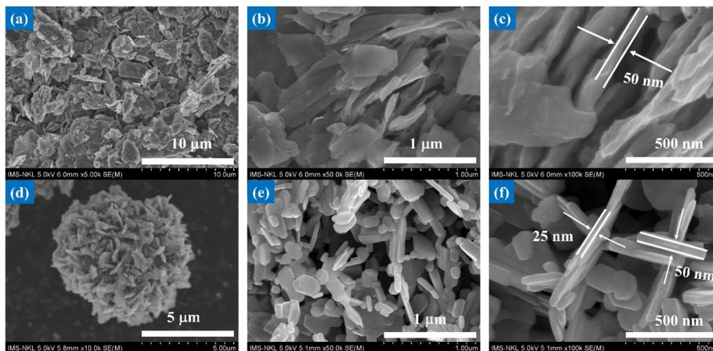
Fig. 1 FE-SEM images at low and high magnifications of different  $V_2O_5$  morphologies: (a)–(c) nanosheets and (d)–(f) flower-like structures composed of nanosheets, obtained after annealing at 500 °C.
