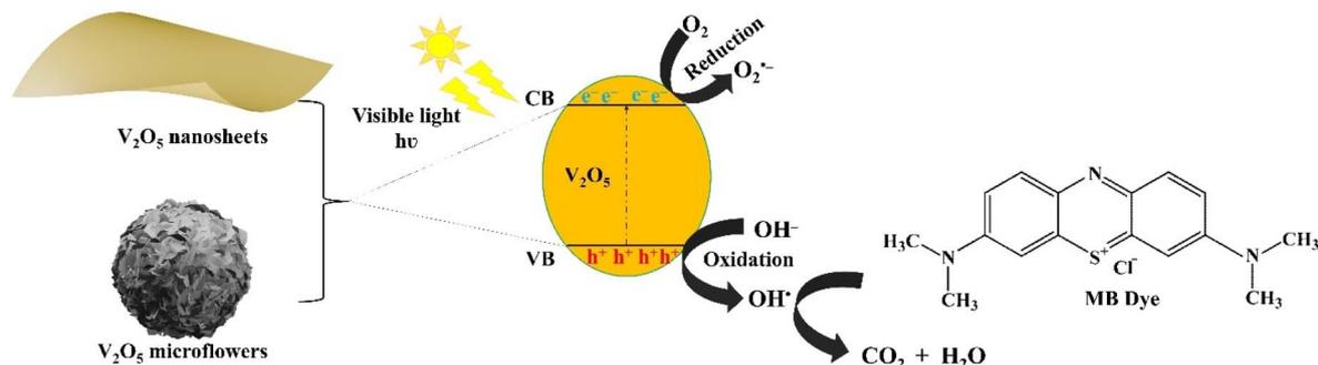
Fig. 12 Photocatalytic degradation mechanism of MB by  $V_2O_5$  nanosheets and microflowers under visible light illumination.
