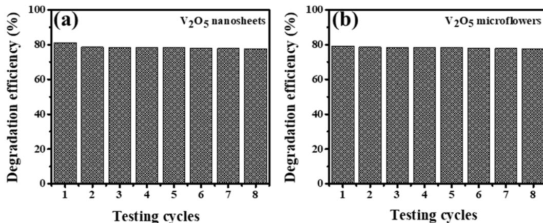
Fig. 9 The stability of (a) V<sub>2</sub>O<sub>5</sub> nanosheets and (b) microflowers photocatalytic activity for the degradation of MB after 60 minutes of light irradiation.
