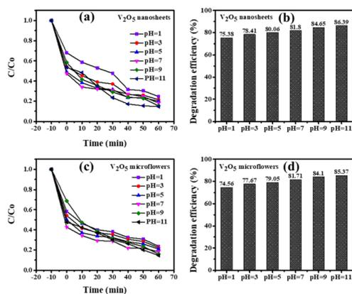
Fig. 10 The effect of pH solutions on the photodegradation of MB by (a) and (b) V<sub>2</sub>O<sub>5</sub> nanosheets and (c) and (d) microflowers photocatalysts after 60 minutes of light irradiation.
