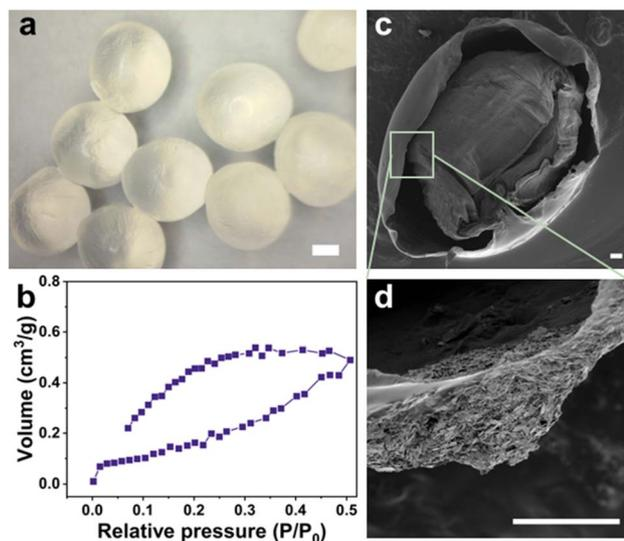
Fig. 2 (a) Optical microscopy image (scale bar = 1 mm), and (b)  $N_2$  adsorption–desorption isotherms of the freeze-dried ALG-as-made beads; SEM images (scale bar =  $100\ \mu\text{m}$ ) of (c) a cross-section and (d) a single inner layer of the freeze-dried beads.
