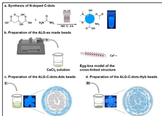
**Scheme 1** Schematic diagram of (a) the synthesis route of the fluorescent C-dots *via* the hydrothermal method; (b) the preparation of pure alginate hydrogel beads and the  $\text{Ca}^{2+}$ -induced cross-linking, (c) and (d) two distinct scenarios investigated in this work for immobilising the fluorescent C-dots on alginate hydrogel systems, named ALG-C-dots-Ads and ALG-C-dots-Hyb, respectively, with different distributions of C-dots and fluorescence within the beads.
