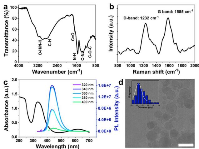
**Fig. 1** (a) FTIR, (b) Raman, and (c) UV-vis absorbance and PL intensity spectra of prepared C-dots; (d) TEM image (scale bar 50 nm) with size distribution of synthesised C-dots, the mean diameter of the C-dots was determined as  $(32.5 \pm 13.0)$  nm, based on a fitted Gaussian model.
