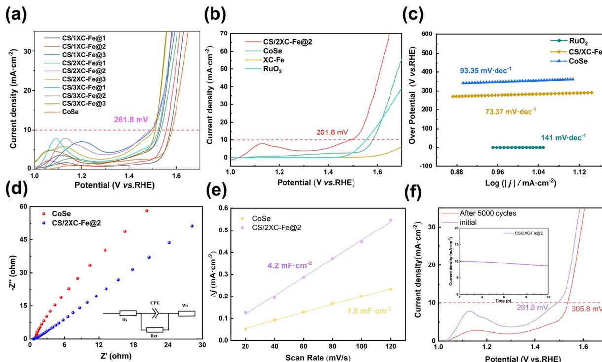
Fig. 3 (a and b) LSV curves. (c) Tafel plots. (d) Nyquist plot of 261.8 mV vs. RHE (for OER). (e) Double-layer capacitance. (f) The LSV curve of CS/2XC-Fe@2 after 5000 cycles (inset: the  $i-t$  curve of  $10 \text{ mA cm}^{-2}$  in OER).
