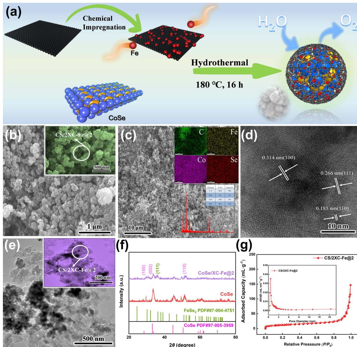
Fig. 1 (a) Schematic diagram of the preparation for CS/yXC-Fe@X, (b) SEM images of CS/2XC-Fe@1 and (c) EDS, (d) and (e) HRTEM and TEM images of CS/2XC-Fe@1, (f) XRD patterns of as-prepared CS/2XC-Fe@1, CoSe, (g) BET of CS/2XC-Fe@2.
