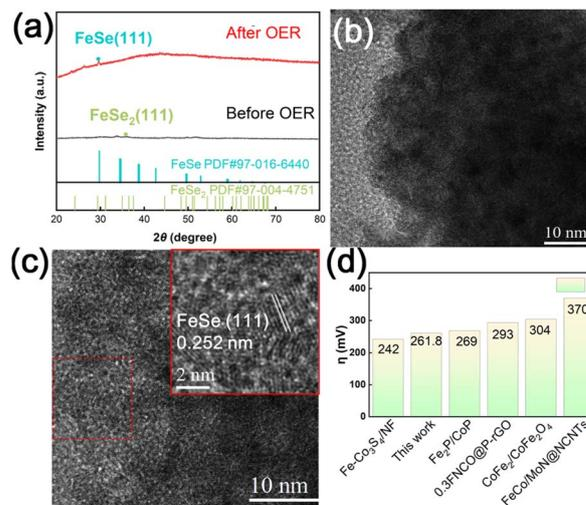
Fig. 4 (a) XRD of CS/2XC-Fe@2 after OER test, (b and c) TEM of CS/2XC-Fe@2 after OER test, (d) bimetallic site OER catalysts in recent studies.<sup>36–38</sup>
