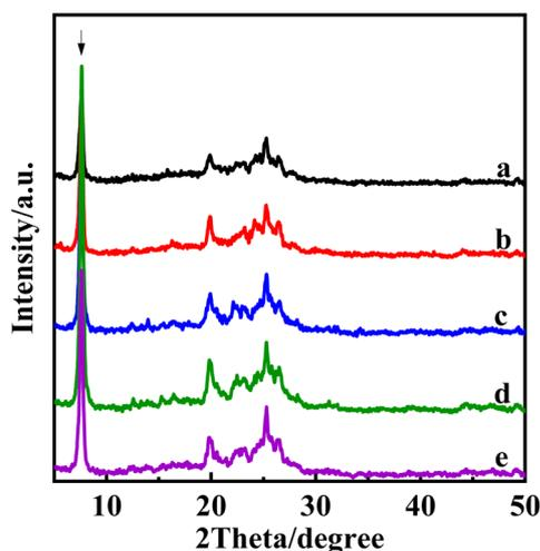
Fig. 5 XRD plots of PLS-1 intercalated using TEOAH, at different times 2 h (a), 4 h (b), 6 h (c), 8 h (d), 10 h (e).
