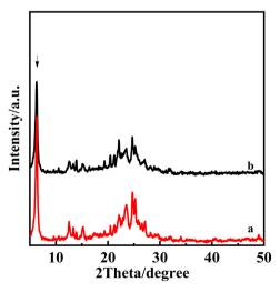
Fig. 6 XRD plots of PLS-1 intercalation using TBAOH under different conditions PLS-1-0.5TBAOH 373 K 8 h (a), PLS-1-TBAOH 373 K 8 h (b).
