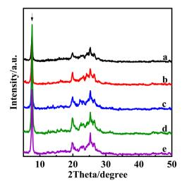
Fig. 5  $\,$  XRD plots of PLS-1 intercalated using TEAOH, at different times 2 h (a), 4 h (b), 6 h (c), 8 h (d), 10 h (e).
