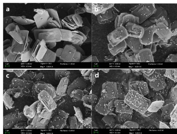
**Fig. 8** SEM image of PLS-1 (a), PLS-1-acid-0.1HE-333-8 (b), PLS-1-0.5TBAOH (c), PLS-1-2Si (d).
