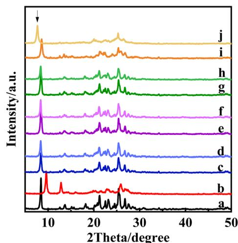
Fig. 3 XRD plots of PLS-1 parent and various post-treatment materials: PLS-1 (a), PLS-1-cal (b), PLS-1-acid-0.1HE-423-0.5 (c), PLS-1-acid-0.1HE-423-0.5-TEAOH (d), PLS-1-acid-0.1HE-423-0.75 (e), PLS-1-acid-0.1HE-423-0.75-TEAOH (f), PLS-1-acid-0.1HE-423-1 (g), PLS-1-acid-0.1HE-423-1-TEAOH (h), PLS-1-acid-0.1HE-423-2 (i), PLS-1-acid-0.1HE-423-2-TEAOH (j).
