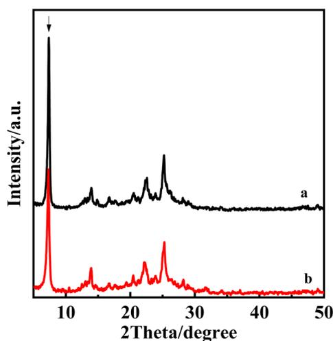
Fig. 9 XRD patterns of interlayer expanded materials using TBAOH-intercalated material as parent with different conditions, PLS-1-2Si-1M HE-443-20 (a), PLS-1-2Si-2M HCl-443-20 (b).
