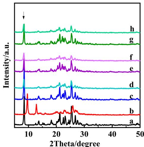
Fig. 2 XRD plots of PLS-1 parent and various post-treated materials: PLS-1 (a), PLS-1-cal (b), PLS-1-acid-0.1H-RT-4 (c), PLS-1-acid-0.1H-RT-4-TEAOH (d), PLS-1-acid-0.1H-333-4 (e), PLS-1-acid-0.1H-333-4-TEAOH (f), PLS-1-acid-0.1H-353-4 (g), PLS-1-acid-0.1H-353-4-TEAOH (h).
