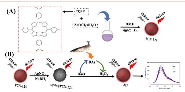
Fig. 1 (A) Preparation of PCN-224. (B) Schematic of AgNPs@PCN-224 for constructing a biosensor to detect histamine.
