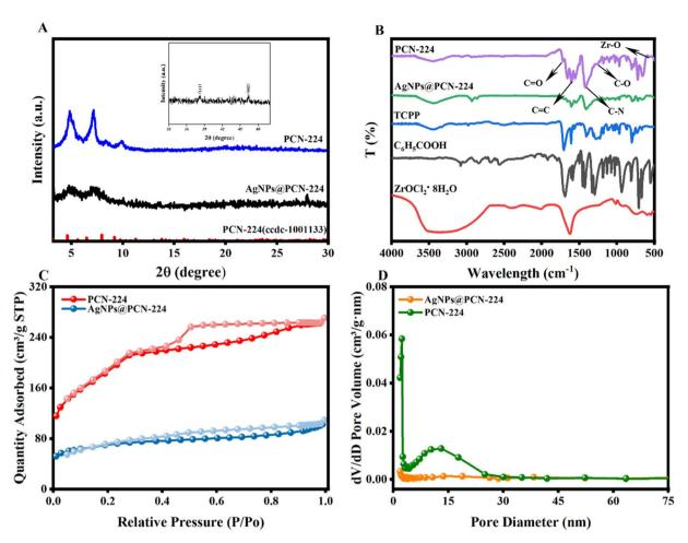
Fig. 3 (A) X-ray diffraction patterns, (B) Fourier transform infrared spectroscopy (FTIR) spectra, (C) N₂ adsorption–desorption isotherms, and (D) pore size distribution diagrams of PCN-224 and AgNPs@PCN-224.
