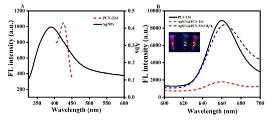
Fig. 5 (A) UV-vis spectrum of AgNPs and fluorescence emission spectrum of PCN-224. (B) Fluorescence spectra of PCN-224 and AgNPs@PCN-224 before and after  $H_2O_2$  was added; inset shows physical drawings of the samples under UV lamp irradiation, marked as 1, 2, and 3, respectively.
