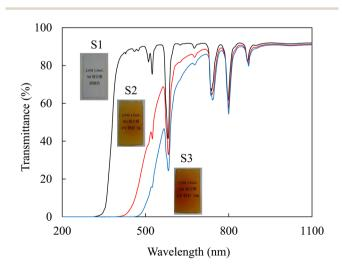
$\label{eq:Fig.1} \textbf{Fig. 1} \quad \textbf{Transmission spectra and photographs of the composite films}.$
