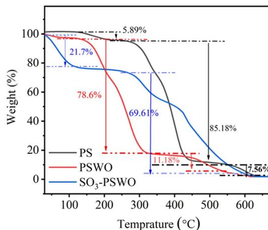
Fig. 6 Thermal stability analysis of PS, PSWO, and SO<sub>3</sub>-PSWO.
