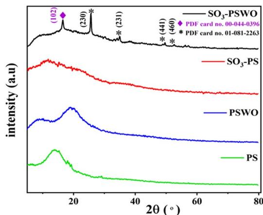
Fig. 5 XRD patterns of PS, PSWO, SO<sub>3</sub>-PS, and SO<sub>3</sub>-PSWO.
