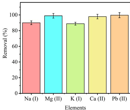
Fig. 10 Effect of interfering ions on  $\text{Pb}^{2+}$  adsorption by  $\text{SO}_3\text{-PSWO}$  ( $C_0 = 100 \text{ mg L}^{-1}$ , S : L ratio  $0.5 \text{ g L}^{-1}$ , pH = 5.5, contact time = 1 hour).
