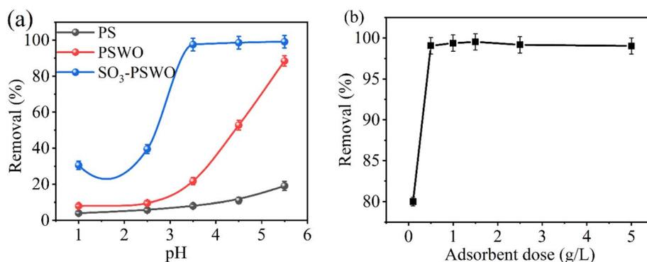
Fig. 7 (a) Effect of pH ranging from 1 to 5.5 on adsorption of Pb<sup>2+</sup> onto PS, PSWO, and SO<sub>3</sub>-PSWO and (b) effect of adsorbent dose in the range of 0.1 to 5 g L<sup>-1</sup> on adsorption efficiency of the SO<sub>3</sub>-PSWO (C<sub>0</sub> = 100 mg L<sup>-1</sup>, S : L ratio = 0.5 g L<sup>-1</sup>, contact time = 1 hour, shaking speed = 250 rpm).
