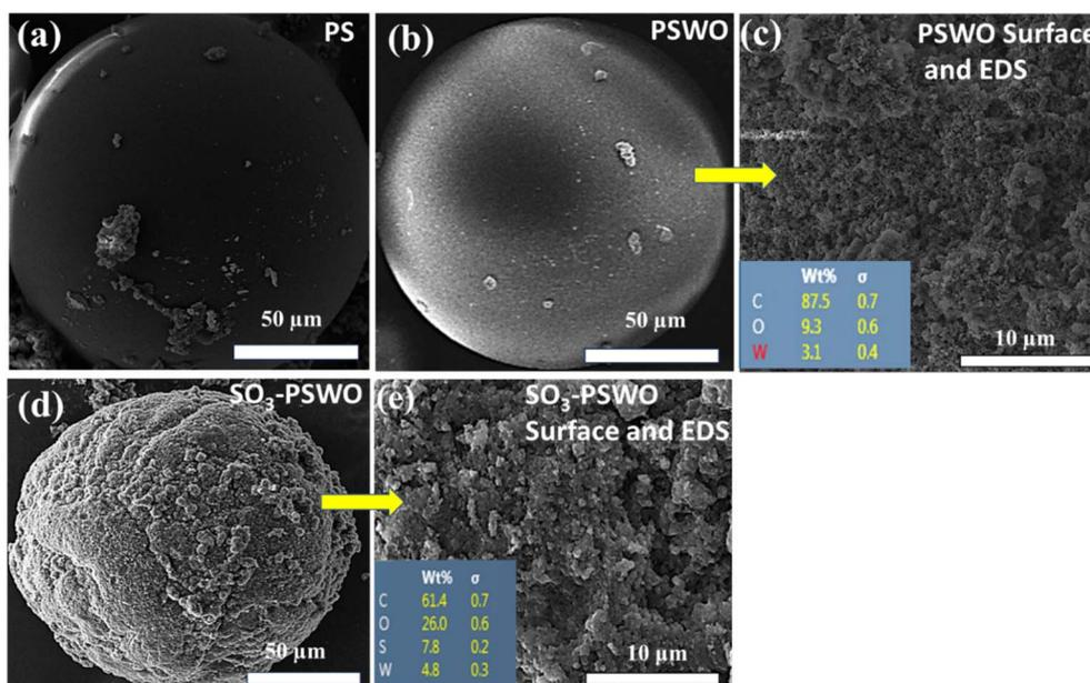
Fig. 4 SEM images of (a) PS and (b) PSWO, (c) the surface of PSWO bead along with its EDS spectrum, and (d and e) the SEM images of SO<sub>3</sub>-PSWO at low and higher magnifications along with EDS data, respectively.
