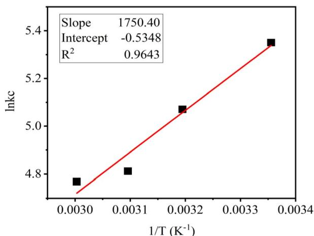
**Fig. 9** ln(k<sub>c</sub>) versus 1/T for Pb<sup>2+</sup> adsorption onto SO<sub>3</sub>-PSWO to determine the change in enthalpy and entropy (C<sub>0</sub> = 100 mg L<sup>-1</sup>, S : L ratio 0.5 g L<sup>-1</sup>, pH = 5.5, contact time = 1 hour).
