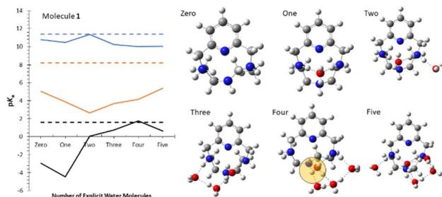
Fig. 4 Explicit solvent calculations for molecule 1. (left) First (blue), second (red), and third (black)  $pK_a$ . Horizontal dashed lines are experimental values, other lines are calculations with 0–5 explicit water molecules. (right) Computed structures for charge +2 state with 0–5 explicit water molecules.
