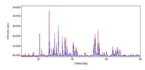
Fig. 2 XRD result of IREM material (red), standard of MP titanium oxide (blue), and standard of potassium titanium oxide (green). The sheet electrode was made of the same material.
