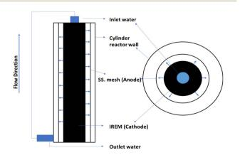
Fig. 1 Reactor setup. The solution containing bromate ions was fed into the reactor at the top inlet, and the permeate solution was collected/re-fed to the reactor at the bottom.
