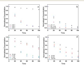
Fig. 5 Effect of (a) different cell voltage, (b) pH, (c) initial bromate concentration, and (d) electrolyte concentration (NaClO<sub>4</sub>). Concentration is normalized to the initial concentration in the solution. Time is in minutes.
