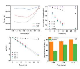
Fig. 3 (a) LSV analysis of bromate ions reduction with various concentrations at sheet electrode (100 mM  $\rm KH_2PO_4$ ), (b) effect of electrode potential (vs. Ag/AgCl) (c) kinetic pseudo-first-order rate at different electrode potential, and (d) effect of atomic hydrogen scavenger at -0.5, -1.0, and -1.5 V vs. Ag/AgCl. Concentrations are expressed relative to the measured initial concentration for each trial. Time is in minutes.
