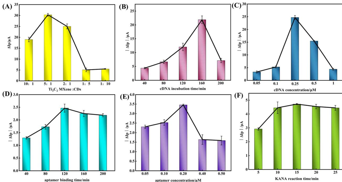
Fig. 4 Effect of (A) the volume ratio of  $\text{Ti}_3\text{C}_2$  MXene to CDs; (B) the cDNA incubation time; (C) the cDNA concentration; (D) the aptamer binding time; (E) the aptamer concentration; (F) the KANA reaction time. The shift of peak current ( $\Delta I_p$ ) was obtained by subtracting the current of the previous modification step. The error bars represented the standard deviation for three repeated measurements.
