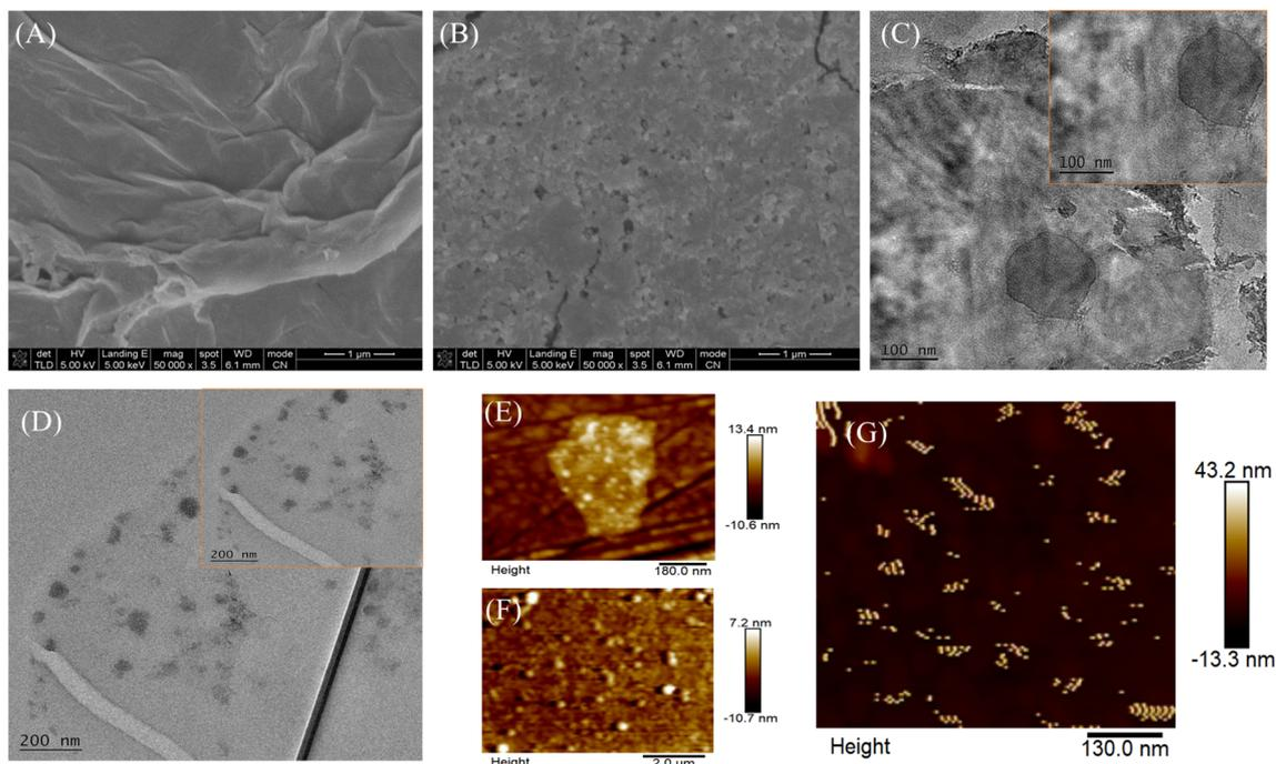
Fig. 1 SEM images of (A)  $\text{Ti}_3\text{C}_2$  MXene and (B)  $\text{CDs@Ti}_3\text{C}_2$  MXene; TEM images of (C)  $\text{Ti}_3\text{C}_2$  MXene and (D)  $\text{CDs@Ti}_3\text{C}_2$  MXene (inset: a cropped section of the image); AFM images of (E)  $\text{Ti}_3\text{C}_2$  MXene, (F) CDs, and (G)  $\text{CDs@Ti}_3\text{C}_2$  MXene.
