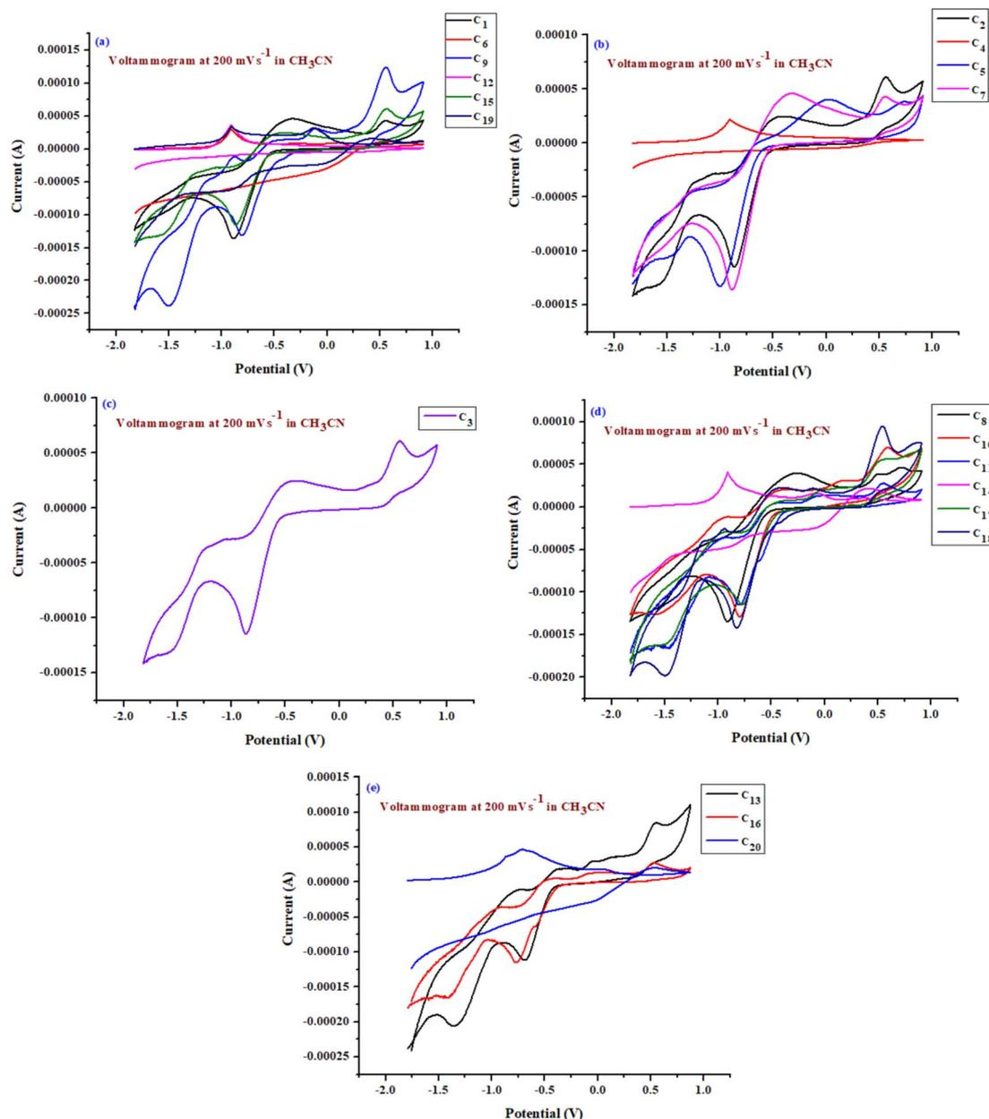
Fig. 3 Comparative cyclic voltammograms based on metal centers (Co, Ni, Fe, Zn and Cu) of all the synthesized TPY-complexes ( $C_1$ – $C_{20}$ ) recorded at a scan rate of  $200 \text{ mV s}^{-1}$ . (a) CV of Co-based TPY complexes. (b) CV of Ni-based TPY complexes. (c) CV of Fe-based TPY complex. (d) CV of Zn-based TPY complexes. (e) CV of Cu-based TPY complexes.
