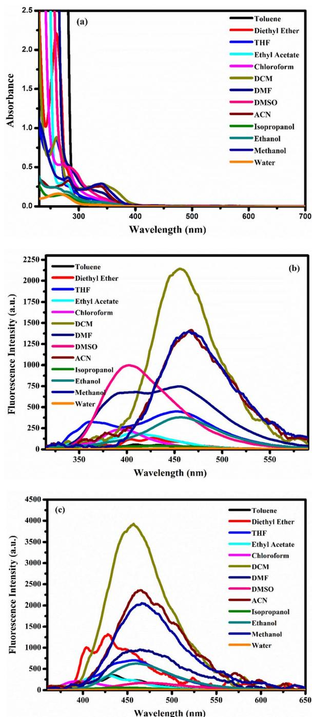
Fig. 2 (a) The UV-vis absorption and (b)  $\lambda_{\text{exc}} = 300$  nm fluorescence spectra and (c)  $\lambda_{\text{exc}} = 350$  nm fluorescence spectra of compound  $C_{18}$  (10  $\mu\text{M}$ ) in different solvents.
