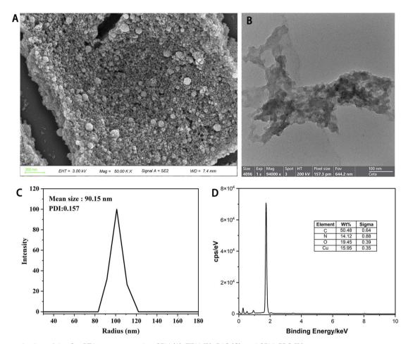
Fig. 1 Characterization of the Cu-PTA nanozyme using SEM (A), TEM (B), DLS (C), and SEM-EDS (D).
