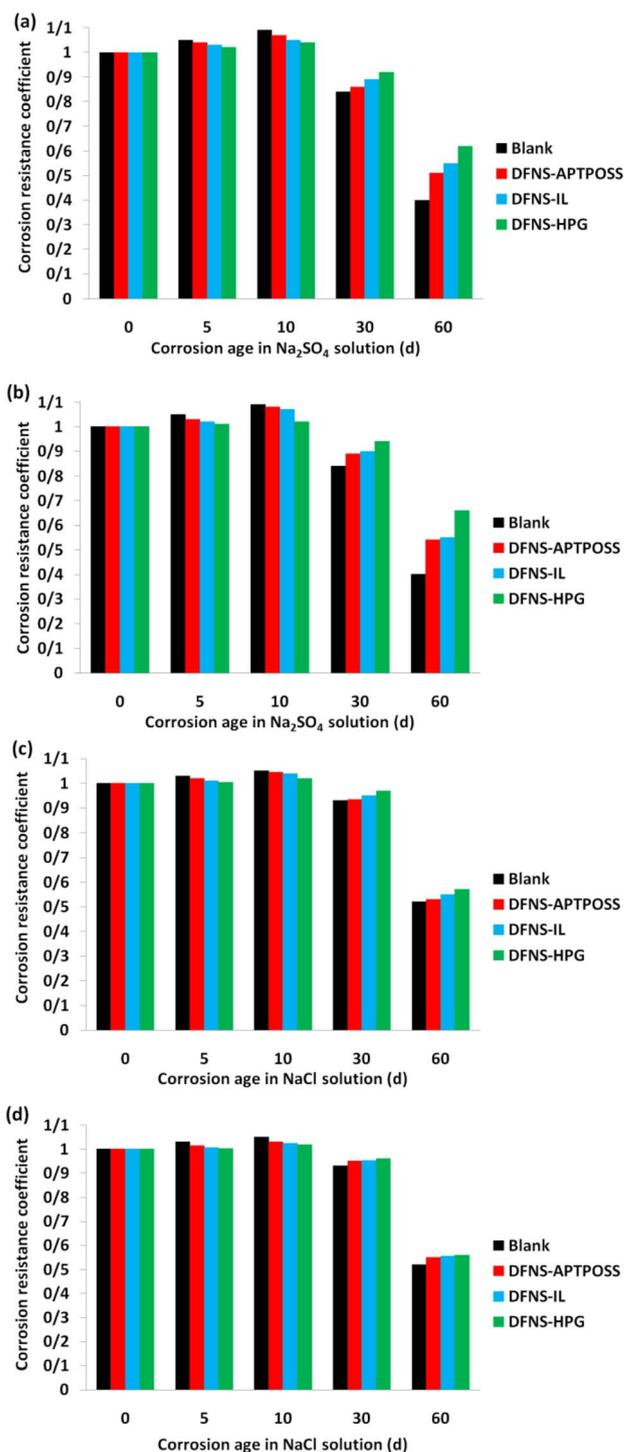
Fig. 11 Corrosion resistance coefficients of cement mortar containing polymers over aging time in an 8% Na<sub>2</sub>SO<sub>4</sub> solution, evaluated based on flexural strength (a) and compressive strength (b); corrosion resistance coefficients of cement mortar containing polymers over aging time in an 8% NaCl solution, evaluated based on flexural strength (c) and compressive strength (d).
