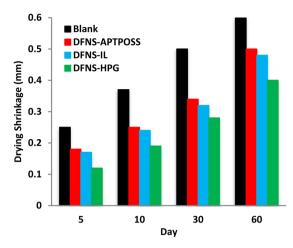
Fig. 15 The effect of different mass fractions on the drying shrinkage of concrete
