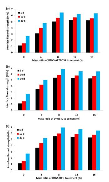
Fig. 10 Interface flexural strengths of cement mortar with polymer specimens with (a) DFNS-APTPOSS, (b) DFNS-IL, and (c) DFNS-HPG.
