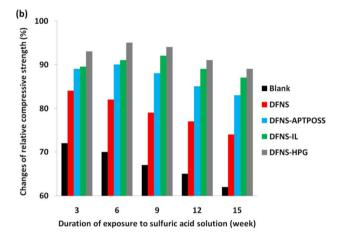
Fig. 17 (a) Relative weight variations and (b) relative compressive strength changes of concrete samples incorporating DFNS-polymers after exposure to sulfuric acid.
