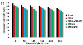
Fig. 16 (a) Weight loss comparison of concrete samples incorporating DFNS, DFNS-APTPOSS, DFNS-IL, and DFNS-HPG after freeze-thaw cycles; (b) compressive strength variations of samples subjected to different freeze-thaw cycles.
