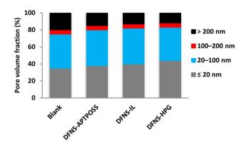
Fig. 13 Pore size distribution of the mortar samples
