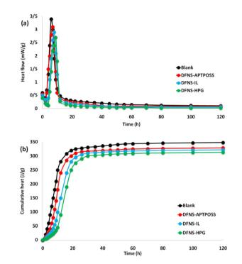
Fig. 5 Heat flow profiles (a) and cumulative heat release profiles (b) of cement pastes incorporating various DFNS-polymers.
