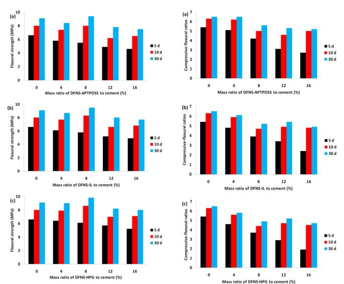
Fig. 8 Flexural strengths of cement mortar with polymer specimens with DFNS-APTPOSS (a), DFNS-IL (b), and DFNS-HPG (c).
