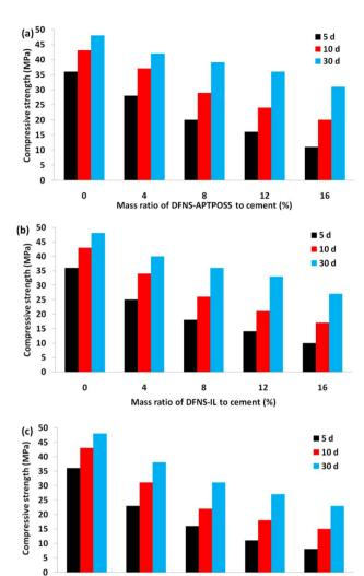
Fig. 7 Compressive strengths of cement mortar with polymer specimens with (a) DFNS-APTPOSS, (b) DFNS-IL, and (c) DFNS-HPG.
