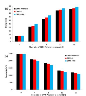
Fig. 6 Slump (a) and apparent densities (b) of cement mortar with polymer based with different DFNS-polymers contents.
