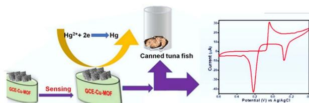
Fig. 9 An illustration of the electrochemical determination of Hg<sup>2+</sup> in tuna fish at Cu-MOF NP-modified electrode. Reproduced from ref. 123 with permission from Elsevier, copyright 2020.
