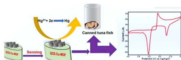
Fig. 9 An illustration of the electrochemical determination of Hg 2+ in tuna fish at Cu-MOF NP-modified electrode. Reproduced from ref. 123 with permission from Elsevier, copyright 2020.
