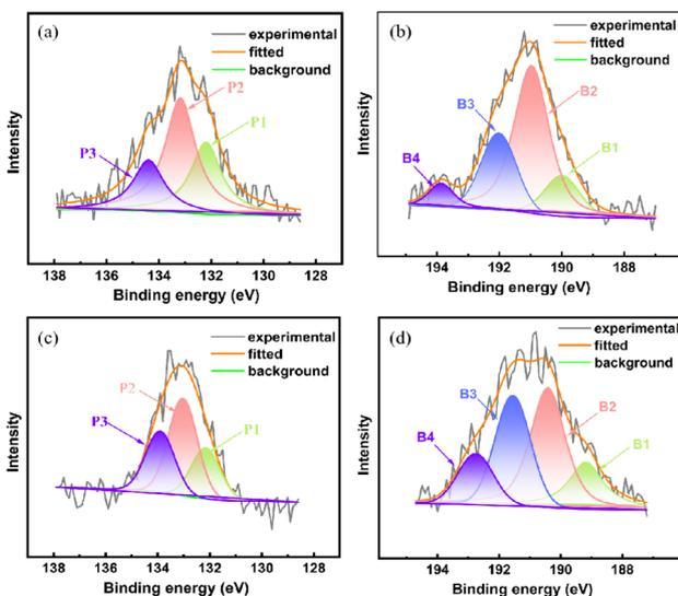
Fig. 5 XPS spectra of P 2p for (a) CNF-N,P, (c) CNF-N,P,B and B 1s for (b) CNF-N,B, (d) CNF-N,P,B.
