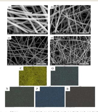
Fig. 1 SEM images of (a) CNF-N, (b) CNF-N,P, (c) CNF-N,B, (d) CNF-N,P,B and EDS mappings of C, O, N, P, and B for CNF-N,P,B.
