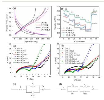
Fig. 6 (a) charge–discharge curves of the third cycles, (b) rate performance (the unit of current densities is A  $g^{-1}$ ), (c) EIS curves of different samples, (d) EIS comparison before and after test for CNF–N and CNF–N,P,B (the lines are the fitted results according to the data points), the equivalent circuits of (e) before test, (f) after test.
