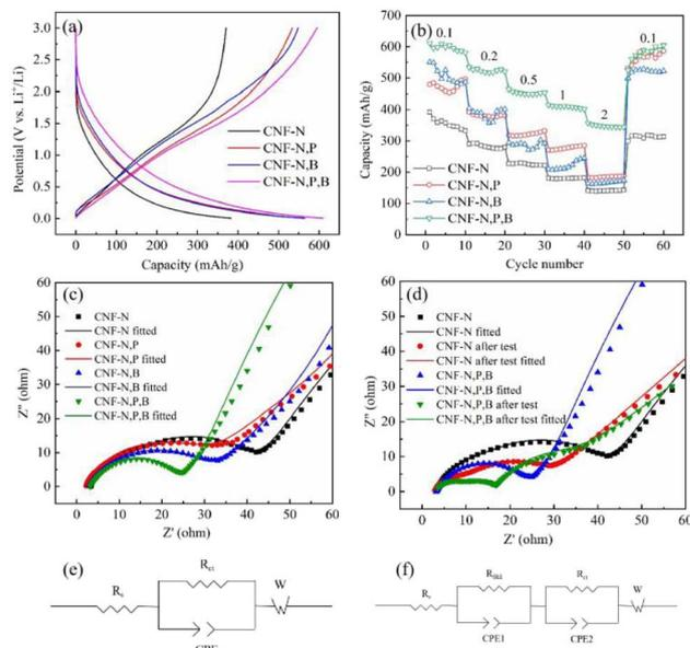
Fig. 6 (a) charge-discharge curves of the third cycles, (b) rate performance (the unit of current densities is A g<sup>-1</sup>), (c) EIS curves of different samples, (d) EIS comparison before and after test for CNF-N and CNF-N,P,B (the lines are the fitted results according to the data points), the equivalent circuits of (e) before test, (f) after test.
