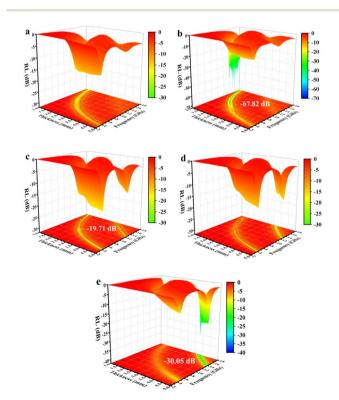
Fig. 7 The 3D reflection loss patterns of mPM: mPM-0.5 (a), mPM-1 (b), mPM-1.5 (c), and mPM-2 (d) and the 3D reflection loss patterns of mesoporous PPy/MXene/Fe $_{7}O_{4}$  (e).
