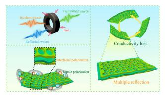
Fig. 13 Mechanism of wave absorption in mPM.
