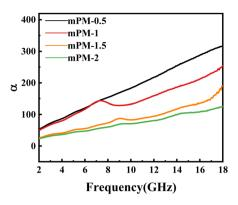
Fig. 11 The plot of attenuation constant  $\alpha$  versus frequency for mPM
