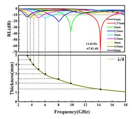
Fig. 12  $\lambda/4$  wavelength matching model of mPM-1.
