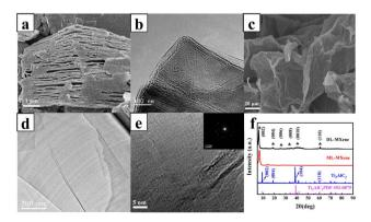
Fig. 2 SEM images of ML-MXene (a) and DL-MXene (c). TEM images of ML-MXene (b) and DL-MXene (d). HRTEM (e) and SAED patterns (inset) of DL-MXene. XRD patterns of DL-MXene, ML-MXene, and Ti<sub>3</sub>AlC<sub>2</sub> (f).
