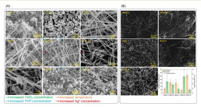
Fig. 5 (A) Factors influence Ag NWs morphology. The optimal Ag NWs morphology is obtained in #NW-2 with synthesis parameters: 20 mM Ag<sup>+</sup> 5 μM FeCl<sub>3</sub>, 200 mM PVP and heated for 150 °C/8 h, while other experiments reveal the effects of parameter change on morphology. (B) SEM images for determining the length of Ag NWs samples, 50 nanowires were measured for every sample.
