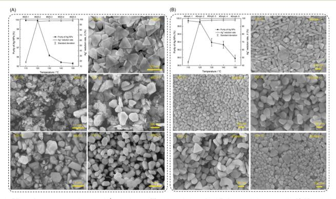
Fig. 6 Effects of temperature on the purity,  $Ag^{+}$  reduction rate (R), and morphology of Ag NPs from crude Ag prepared by ES-PR method with PVP addition. The elevated reaction temperature increased the reducibility of ethylene glycol solution, resulting in an increased R and decreased Ag NPs purity. The morphologies of Ag NPs differ depending on the chemical compositions of crude Ag, indicating that impurity ions play a critical role in morphology control. (A) 925-Ag. (B) Smelt.-Ag.
