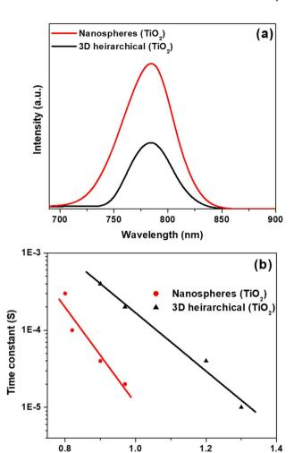
Fig. 4 (a) Steady-state PL spectra of perovskite absorber film coated on  ${\rm TiO_2}$  nanostructures, and (b) electron lifetime for the corresponding nanostructures.
