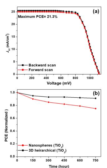
Fig. 5 (a) J-V curves (in reverse and forward scans) of the best-performing cell based on TiO $_2$  3D hierarchical structure and (b) long-term stability test for cells made with TiO $_2$  nanospheres and TiO $_2$  3D hierarchical structures.
