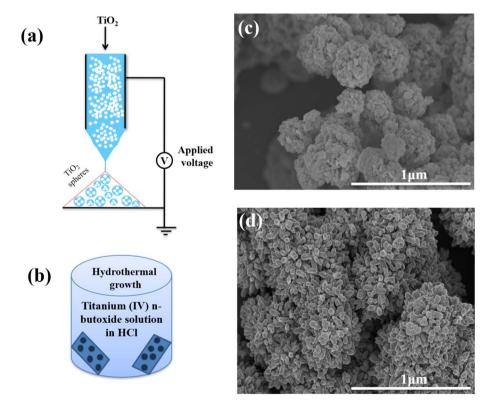
Fig. 1 Schematic of (a)  $TiO_2$  nanospheres deposited *via* an electrospray technique, (b)  $TiO_2$  3D hierarchical structure formed *via* a hydrothermal process, and SEM images of (c)  $TiO_2$  nanospheres and (d)  $TiO_2$  3D hierarchical structure.
