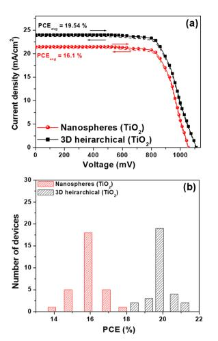
Fig. 3 Assessment of (a) J-V plots of  $TiO_2$  nanospheres and  $TiO_2$  3D hierarchical structure, and (b) bar graphs of the matching cells showing the differences in efficiency for 30 separate cells.
