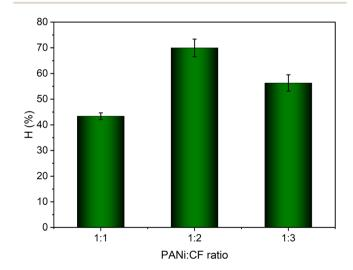
Fig. 3 The effect of the ratio of PANi composition to the CF on  $\mathrm{NH_4}^+$  adsorption efficiency; experimental conditions: initial  $\mathrm{NH_4}^+$  concentration 20 mg  $\mathrm{L^{-1}}$ ; adsorbent dosage 0.6 g  $\mathrm{L^{-1}}$  and pH 7, contact time of 20 min.
