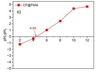
Fig. 2 BET analysis (a), FTIR (b) and pH<sub>PZC</sub> (c) of CF@PANi.
