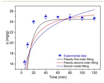
Fig. 8 Kinetic models of  $NH_4^+$  adsorption by CF@PANi.
