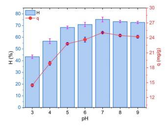
Fig. 4 The effect of pH solution on  $NH_4^+$  adsorption efficiency using CF@PANi; experimental conditions: initial  $NH_4^+$  concentration 20 mg  $L^{-1}$ ; adsorbent dosage 0.6 g  $L^{-1}$ , contact time of 40 min.
