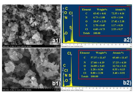
Fig. 1 SEM image and EDS spectra of CF@PANi before (a1 and a2) and after ammonium adsorption (b1 and b2).
