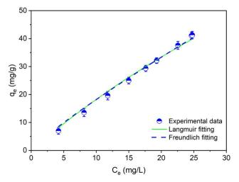
Fig. 9 Ammonium adsorption Isotherm model using CF@PANi.
