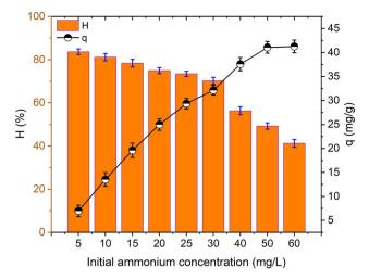
Fig. 7 Effect of  $\mathrm{NH_4}^+$  concentration on adsorption capacity and efficiency using CF@PANi materials, experimental conditions: contact time of 40 min; adsorbent dosage 0.6 g  $\mathrm{L^{-1}}$ , pH 7.
