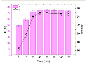
Fig. 5 Effect of contact time on the  $\mathrm{NH_4}^+$  adsorption efficiency using CF@PANi materials; experimental conditions: initial  $\mathrm{NH_4}^+$  concentration 20 mg  $\mathrm{L}^{-1}$ ; adsorbent dosage 0.6 g  $\mathrm{L}^{-1}$ , pH 7.
