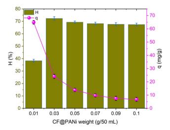
Fig. 6 Effect of CF@PANi weight on the  $NH_4^+$  adsorption efficiency; experimental conditions: initial  $NH_4^+$  concentration 20 mg  $L^{-1}$ ; pH 7 and contact time 40 min.
