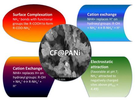
Fig. 10 Ammonium adsorption onto CF@PANi.
