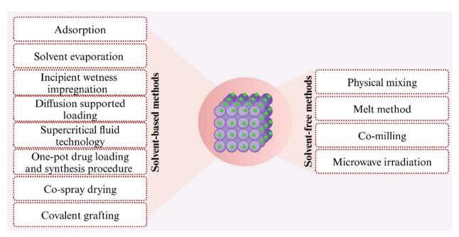
Fig. 6 Schematic of the various approaches utilized to load drugs into MMS NPs based on solvent-free procedures and solvent-based procedures.
