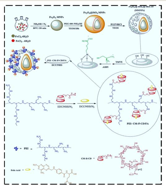
Fig. 2 Synthetic path for the preparation of the targeted MMNPs nanocarrier. Reproduced from ref. 49 with permission from Elsevier, Copyright 2021.
