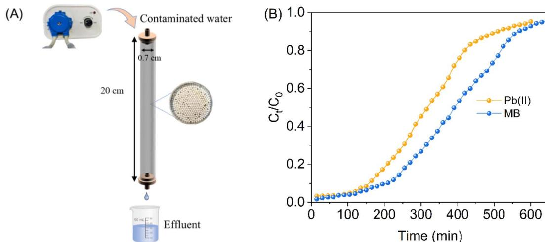
Fig. 9 (A) Schematic of the adsorption fixed-bed mini-column. (B) Adsorption breakthrough curves for  $\text{Pb(II)}$  and  $\text{MB}$ .
