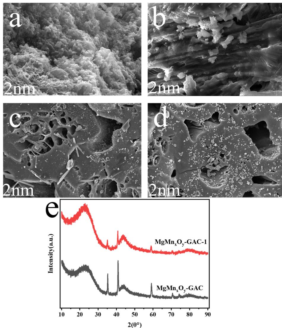
Fig. 5 SEM comparison of Mn-GAC and  $\text{MgMn}_x\text{O}_y\text{-GAC}$  catalysts before and after cationic red degradation. (a and b) Surface morphology before and after Mn-GAC degradation, (c and d) surface morphology of  $\text{MgMn}_x\text{O}_y\text{-GAC}$  before and after degradation, and (e) XRD pattern.
