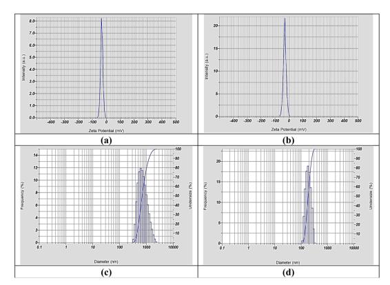
Fig. 3 Zeta potential and DLS analysis: (a) zeta potential of Ag-TiO<sub>2</sub> NC and (b) Ag-SeO<sub>2</sub> NC. (c) DLS of Ag-TiO<sub>2</sub> NC and (d) Ag-SeO<sub>2</sub> NC.
