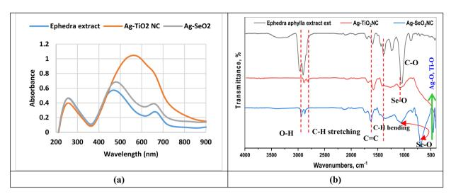
Fig. 2 Spectral analysis of the plant extract and nanocomposites: (a) UV-visible spectra and (b) FTIR spectra of *Ephedra aphylla* extract (23.98 mg mL $^{-1}$ ), Aq-TiO<sub>2</sub> NC (33.16 mg mL $^{-1}$ ), and Aq-SeO<sub>2</sub> NC (18.92 mg mL $^{-1}$ ).
