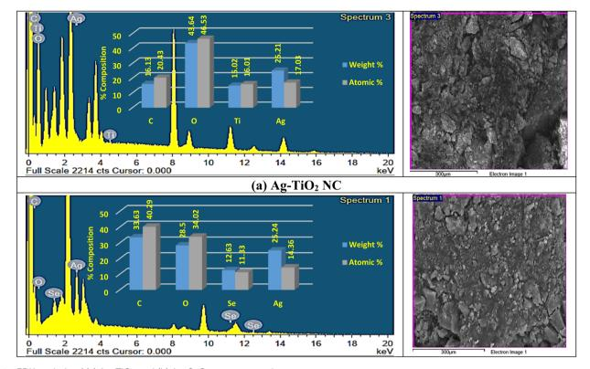
Fig. 5 EDX analysis of (a) Ag-TiO<sub>2</sub> and (b) Ag-SeO<sub>2</sub> nanocomposites.
