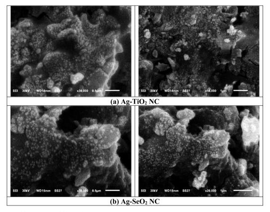
Fig. 6 SEM images of (a) Ag-TiO<sub>2</sub> and (b) Ag-SeO<sub>2</sub> nanocomposites.
