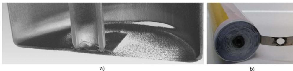
Fig. 4 CT scan of the negative electrode of an 18 650 battery after vibrations: (a) CT image and (b) corresponding photograph.<sup>64</sup>
