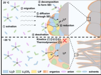
Fig. 3 Schematic of lithium-ion diffusion and charge transfer at room and low temperature. Low temperature not only reduces the speed of Li<sup>†</sup> through the electrolyte and the SEI layer but also leads to incomplete electrolyte decomposition, resulting in the formation of an SEI membrane composed of metastable intermediate products rich in organic matter, which is prone to lithium dendrite growth.<sup>54</sup>
