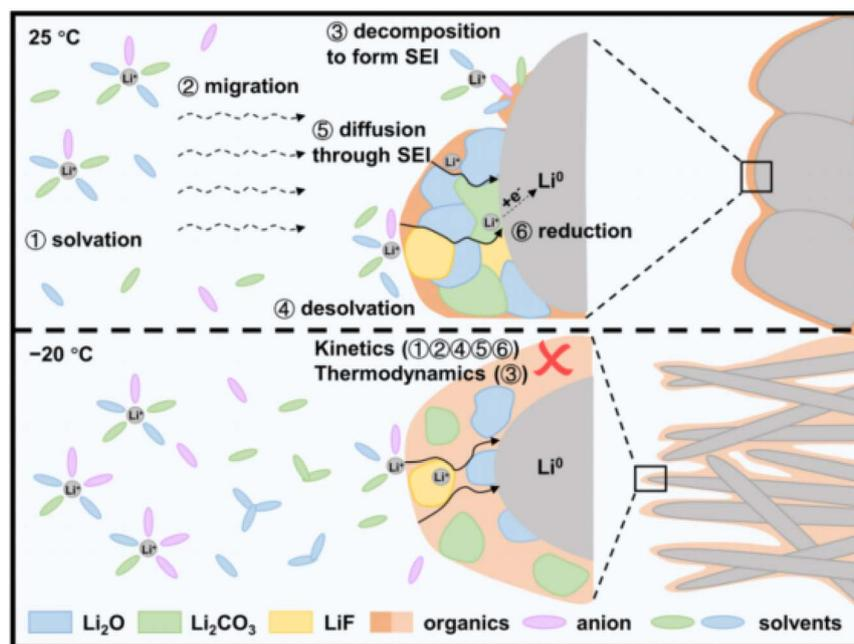
Fig. 3 Schematic of lithium-ion diffusion and charge transfer at room and low temperature. Low temperature not only reduces the speed of  $\text{Li}^+$  through the electrolyte and the SEI layer but also leads to incomplete electrolyte decomposition, resulting in the formation of an SEI membrane composed of metastable intermediate products rich in organic matter, which is prone to lithium dendrite growth.<sup>54</sup>
