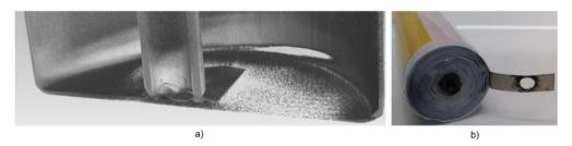
Fig. 4 CT scan of the negative electrode of an 18 650 battery after vibrations: (a) CT image and (b) corresponding photograph.
