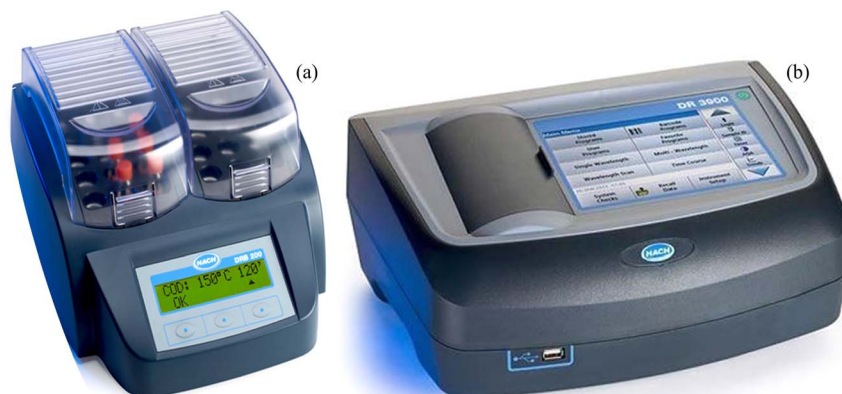
Fig. 2 COD standard value collection equipment. (a) DRB200 digester device; (b) DR3900 visible spectrophotometer.
