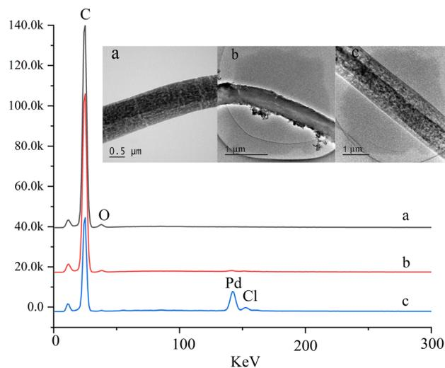
Fig. 3 TEM images and EDX spectra of (a) PS electrospun nanofibres, (b) the PdCl<sub>2</sub> coating PS nanofibres on and (c) Pd(II)/PEI/PS nanofibres.
