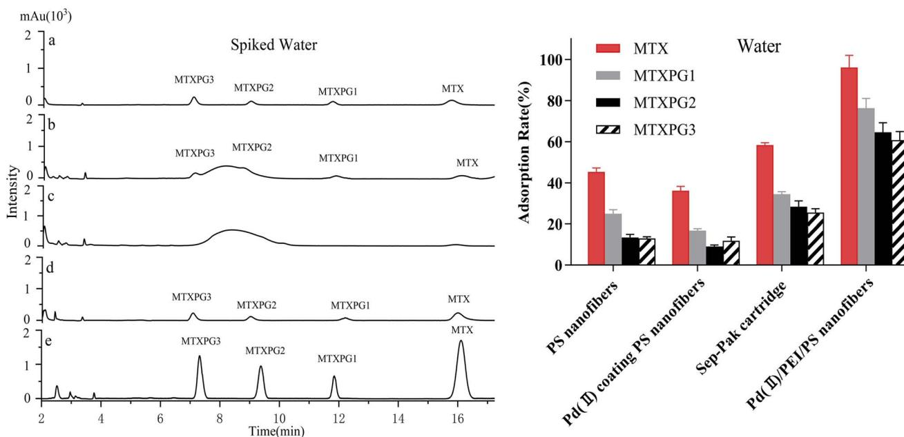
Fig. 6 Left: HPLC chromatograms of spiked water (10 ng/mL), (a) standard solution consisting of MTX and MTXPG1-3, (b) SPE using PS nanofibres, (c) SPE using PdCl<sub>2</sub> coating PS nanofibres, (d) SPE using a conventional Sep-Pak cartridge, and (e) SPE using Pd(II)/PEI/PS nanofibres. Right: The adsorption rate of MTX and MTXPGs in water samples by using PS nanofibres, PdCl<sub>2</sub> coating PS nanofibres, conventional Sep-Pak cartridges and Pd(II)/PEI/PS nanofibres, respectively.
