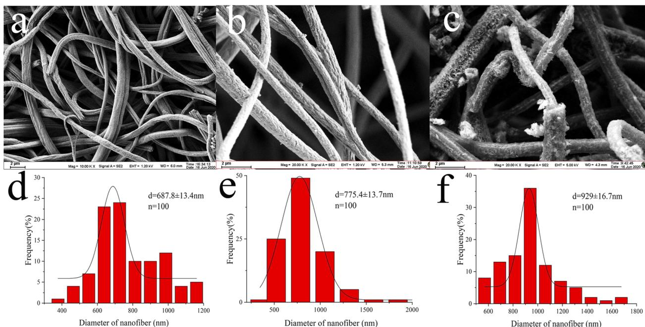
Fig. 2 SEM images of (a) PS electrospun nanofibres, (b) PdCl<sub>2</sub> coating PS nanofibres, and (c) Pd(II)/PEI/PS nanofibres, and the size distribution histogram of (d) PS nanofibres, (e) the PdCl<sub>2</sub> coating PS nanofibres, and (f) Pd(II)/PEI/PS nanofibres.
