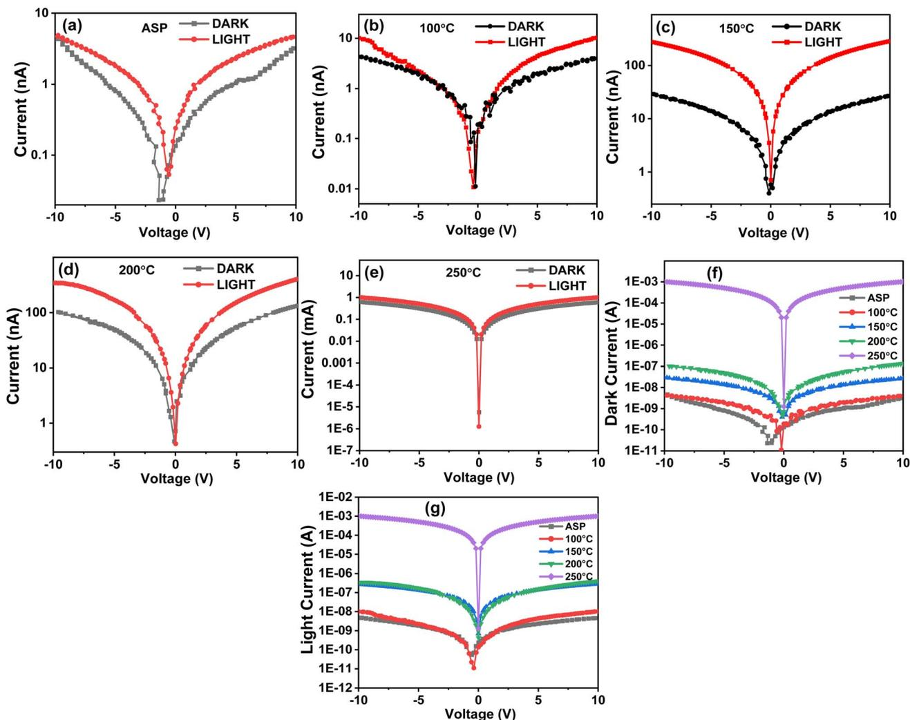
Fig. 9  $I$ - $V$  characteristics plots of as-prepared and annealed  $\text{Ag}_2\text{S}/\text{In}_2\text{Se}_3$  thin films plotted in logarithmic scale for both dark and light conditions (a) asp, (b) 100 °C, (c) 150 °C, (d) 200 °C, (e) 250 °C, combined  $I$ - $V$  plots of all the samples (f) in dark condition and (g) in light condition.
