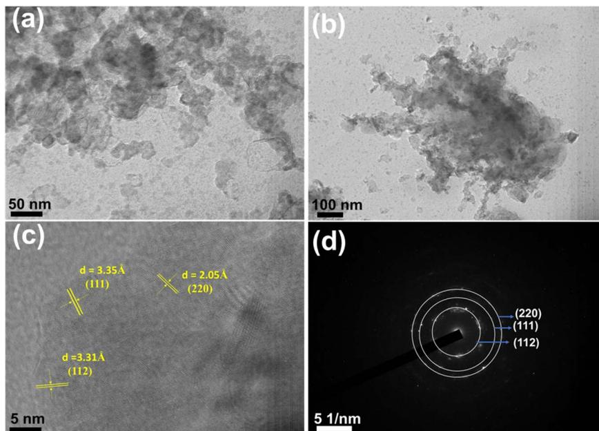
Fig. 5 (a and b) TEM picture, (c) HRTEM picture, and (d) SAED pattern of 250 °C annealed  $\text{Ag}_2\text{Se}/\text{In}_2\text{Se}_3$  thin film.
