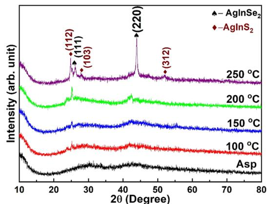
Fig. 1 Structural data by XRD for  $\text{Ag}_2\text{S}/\text{In}_2\text{Se}_3$  films.
