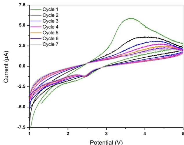
Fig. 6 Linear sweep voltammograms of cycle from 1 to 7 with Li|S-SE|RC 5: CB|stainless steel cell at scan rates of  $100 \mu\text{V s}^{-1}$  from 1 to 5 V vs. Li<sup>+</sup>/Li at RT.
