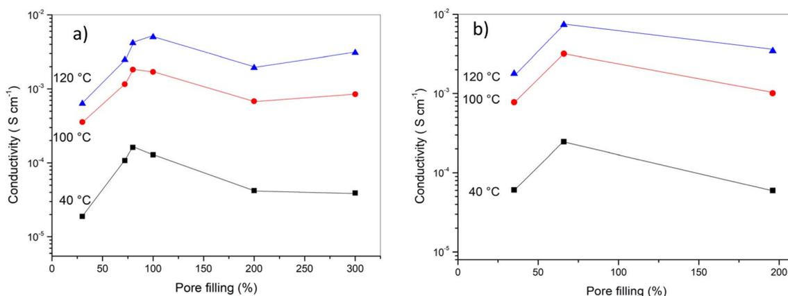
Fig. 5 Li-ion conductivity at 40 °C, 100 °C and 120 °C reported as a function of pore filling, with lines as a guide for the eyes, for (a) samples from RC 1 to RC 6 and for (b) samples from OX 1 to OX 3.
