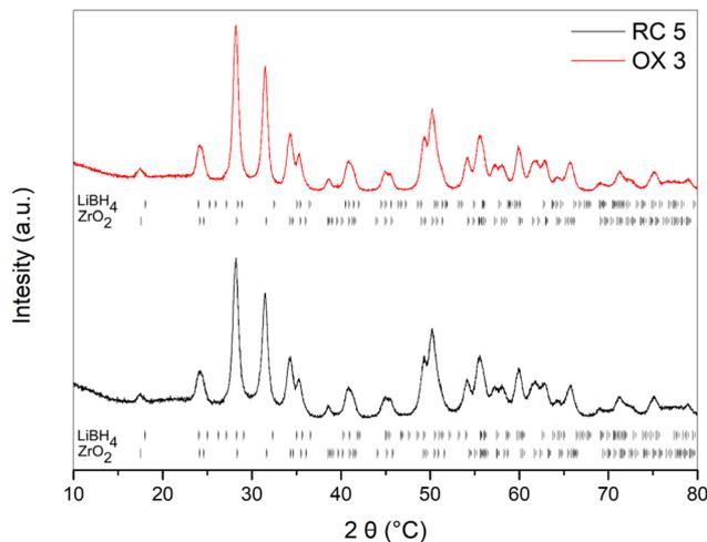
Fig. 2 XRD pattern of samples RC 5 (bottom) and OX 3 (top). Sticks, obtained by Rietveld refinement, show the position of diffraction peaks for both orthorhombic  $\text{LiBH}_4$  (COD code 1504402) and monoclinic  $\text{ZrO}_2$  (COD code 9007485) phases.
