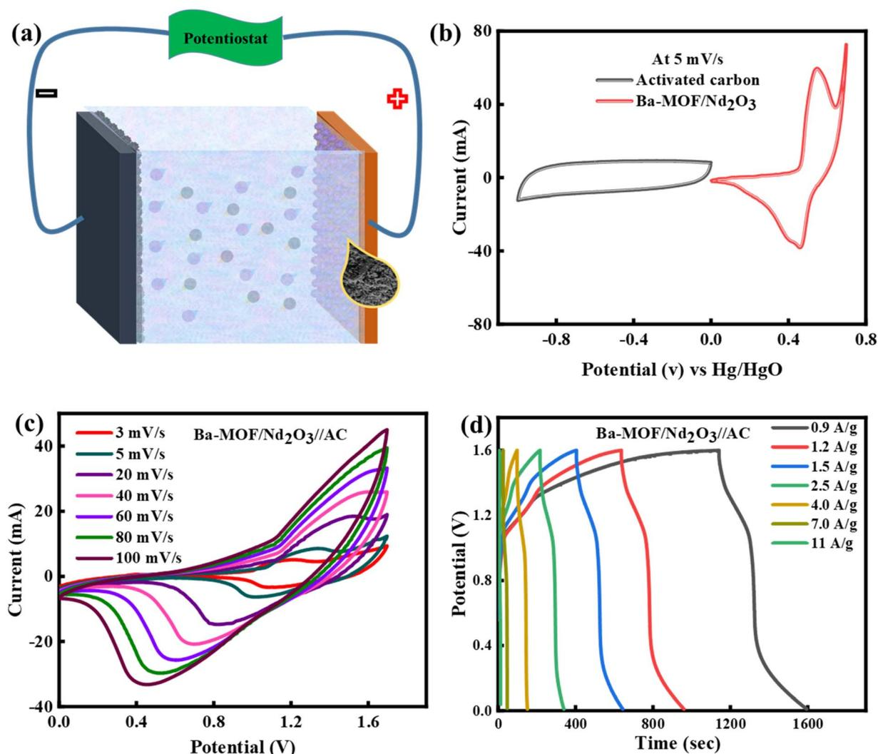
Fig. 6 (a) Schematic of the device. (b) CV curve of both battery grade and capacitive electrodes at 5 mV s<sup>-1</sup> (c) CV graph of the assembled device (Ba-MOF/Nd<sub>2</sub>O<sub>3</sub>//AC). (d) GCD investigation of the device.
