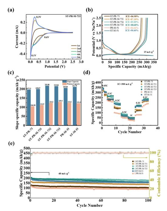
Fig. 5 Electrochemical performance of HCs. (a) CV curves of ST-PR-M-732 in the first three cycles with the scan rate of 0.1 mV s<sup>-1</sup> (b) The first discharge/charge profiles of HCs at 0.05C (15 mA g<sup>-1</sup>). (c) Slope and plateau capacities of HCs at 0.05C (15 mA g<sup>-1</sup>). (d) Discharge capacity at various rates (1C = 300 mA g<sup>-1</sup>). (e) Cycling performance of HCs at 0.2C.
