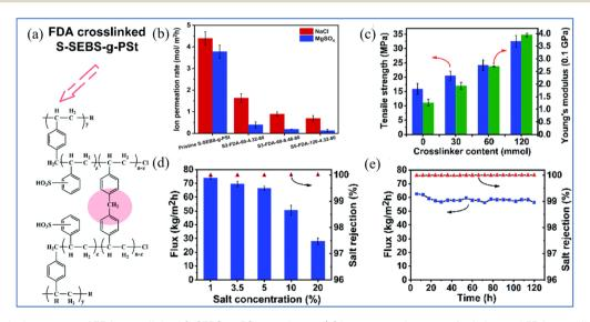
Fig. 12 (a) Chemical structure of FDA-crosslinked S-SEBS-*g*-PSt membrane. (b) Ion permeation rate of pristine and FDA-crosslinked S-SEBS-*g*-PSt membranes. (c) Tensile strength and young's modulus of S-SEBS-*g*-PSt membrane. (d) and (e) Effect of the feed concentration and long term performance of FDA-crosslinked S-SEBS-*g*-PSt membranes (65 °C). Reproduced from ref. 129 with permission from The Royal Society of Chemistry, copyright 2022.
