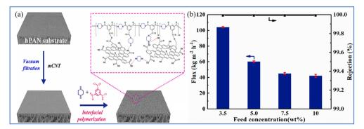
Fig. 11 (a) Illustration of the preparation of PA-mCNT on the hPAN ultrafiltration membrane. (b) Dependance of water flux and salt rejection on feed concentration.<sup>120</sup> Reproduced from ref. 120 with permission from Elsevier, copyright 2022.
