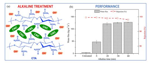
Fig. 8 (a) Illustration of the alkaline treatment of CTA/CNC composite membrane. (b) Dependance of water flux and salt rejection of CTA/CNC composite PV membrane on alkaline treatment time (3.5 wt% NaCl).95 Reproduced from ref. 95 with permission from Elsevier, copyright 2021.
