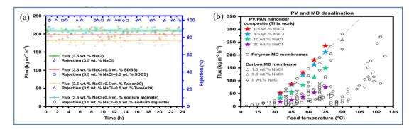
Fig. 5 (a) Water flux and salt rejection of PVA-based composite membrane (3.5 wt% NaCl). (b) Comparing the water flux in this work with other reported publications.<sup>62</sup> Reproduced from ref. 62 with permission from *Nature*, copyright 2020.
