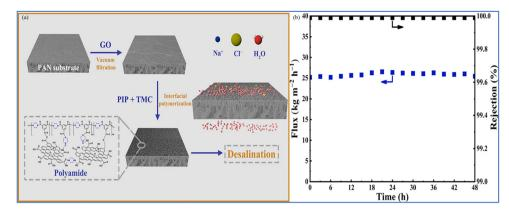
Fig. 2 (a) Illustration of the preparation process of PAG@GO-PA PV composite membranes. (b) Long-term water flux and salt rejection of PAG@GO-PA PV (3.5 wt% NaCl).<sup>54</sup> Reproduced from ref. 54 with permission from American Chemical Society, copyright 2020.
