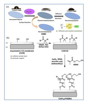
Fig. 7 (a) Diffusion and reaction mechanism of plasma treated polymer membrane.<sup>88</sup> (b) Illustration of the reaction process for surface modification of CAM.<sup>91</sup> Reproduced from ref. 88 and 91 with permission from *Nature* and Elsevier, copyright 2024 and 2024, respectively.
