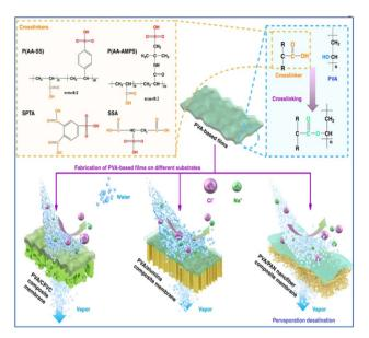
Fig. 4 Illustration of the chemical structures of crosslinkers, crosslinking reaction details and water transport in PV membranes.<sup>62</sup> Reproduced from ref. 62 with permission from Elsevier, copyright 2022.
