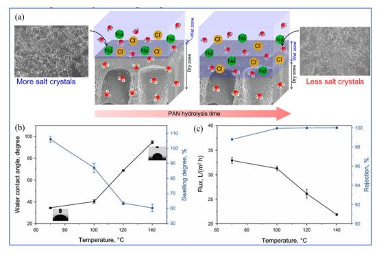
Fig. 9 (a) The proposed mechanism for PV desalination using hydrolyzed PAN porous membranes.<sup>108</sup> (b) The water contact angles and swelling properties. (c) The water flux and salt rejection (using the 35 000 ppm NaCl solution as the feed at 70 °C) of M-d composite membranes crosslinked at different temperatures for 2 h.<sup>109</sup> Reproduced from ref. 108 and 109 with permission from Elsevier, copyright 2019 and 2018.
