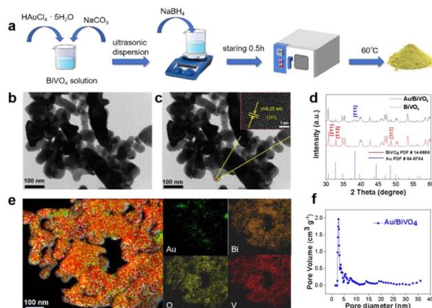
Fig. 1 (a) Schematic for diagram illustrating synthetic procedure of  $\text{Au/BiVO}_4$ . (b) TEM and (c) HR-TEM images of  $\text{Au/BiVO}_4$ . (d) XRD pattern of  $\text{Au/BiVO}_4$ . (e) HAADF-STEM and corresponding elemental mapping images of  $\text{Au/BiVO}_4$ . (f) Pore size distribution curve of  $\text{Au/BiVO}_4$ .
