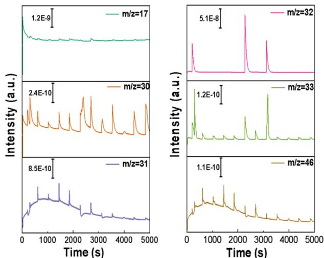
Fig. 4 *In situ* DEMS measurements of NitRR over Au/BiVO<sub>4</sub>.
