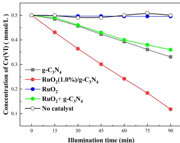
Fig. 7 Photocatalytic reductions of  $\text{Cr}(\text{vi})$  by pure  $g\text{-C}_3\text{N}_4$ , pure  $\text{RuO}_2$  and  $\text{RuO}_2$  (1.0%)/ $g\text{-C}_3\text{N}_4$  composite (solution volume, 200 mL; catalyst, 0.1 g; initial  $\text{Cr}(\text{vi})$  concentration, 0.5 mM; initial pH, 2.3; light source, LED (410 nm, 40 W)).
