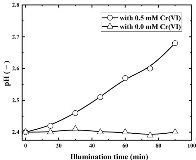
Fig. 9 Variations of pH during illumination with and without Cr(vi) (solution volume, 200 mL; RuO<sub>2</sub> (1.0%)/g-C<sub>3</sub>N<sub>4</sub> composite, 0.1 g; initial Cr(vi) concentration, 0.5 mM; pH<sub>0</sub>, 2.4; light source, LED (410 nm, 40 W)).
