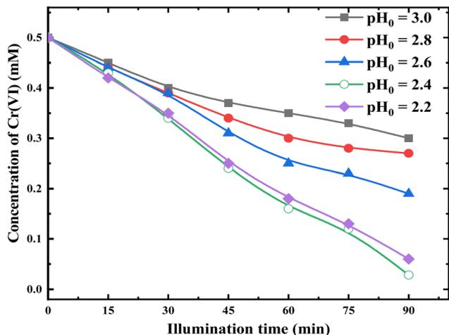
Fig. 8 Photocatalytic reduction of Cr(vi) with RuO<sub>2</sub> (1.0%)/g-C<sub>3</sub>N<sub>4</sub> under different pH<sub>0</sub> values (solution volume, 200 mL; catalyst, 0.1 g; initial Cr(vi) concentration, 0.5 mM; light source, LED (410 nm, 40 W)).
