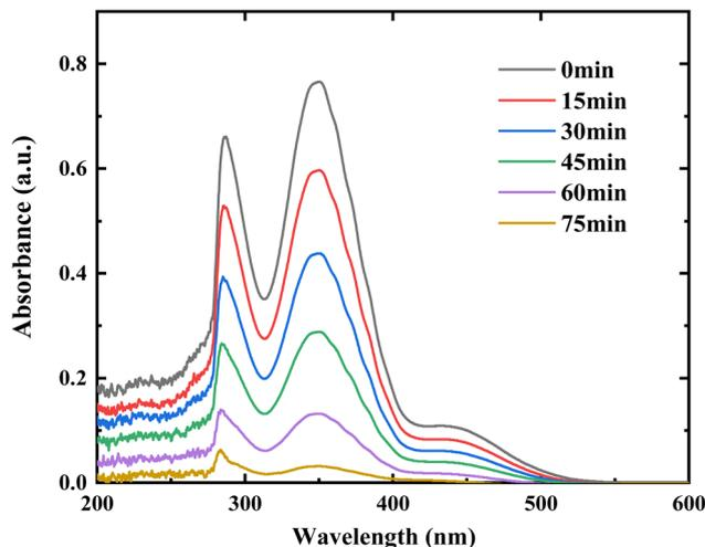
Fig. 12 Evolution of UV-Vis absorption spectra of the solution during photocatalytic reduction of Cr(vi) (solution volume, 200 mL; RuO<sub>2</sub> (1.0%)/g-C<sub>3</sub>N<sub>4</sub> composite, 0.1 g; initial Cr(vi) concentration, 0.5 mM; pH<sub>0</sub>, 2.4; light source, LED (410 nm, 40 W)).
