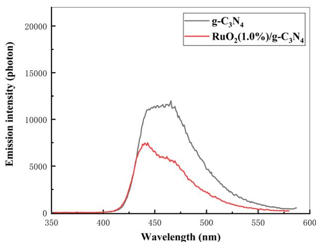
Fig. 13 Fluorescence emission spectra of g-C<sub>3</sub>N<sub>4</sub> and RuO<sub>2</sub> (1.0%)/g-C<sub>3</sub>N<sub>4</sub>.
