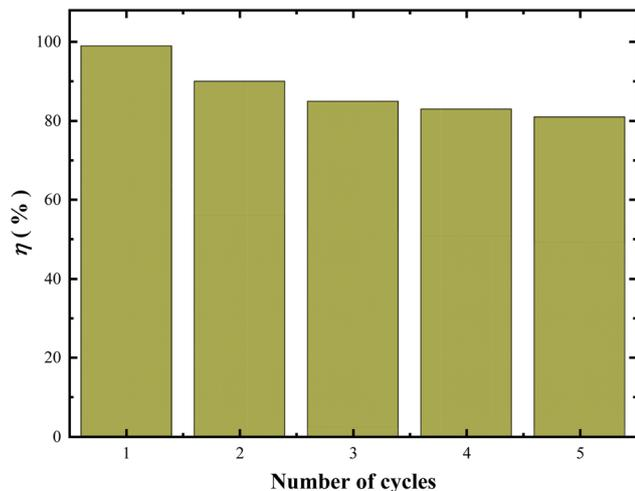
**Fig. 16** Cycle stability test of RuO<sub>2</sub> (1.0%)/g-C<sub>3</sub>N<sub>4</sub> composite (solution volume, 200 mL; RuO<sub>2</sub> (1.0%)/g-C<sub>3</sub>N<sub>4</sub> composite, 0.1 g; initial Cr(VI) concentration, 0.5 mM; pH<sub>0</sub>, 2.4; light source, LED (410 nm, 40 W)).
