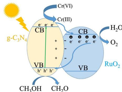
Fig. 14 Mechanism of photocatalytic reduction of Cr(vi) by RuO<sub>2</sub>/g-C<sub>3</sub>N<sub>4</sub>.
