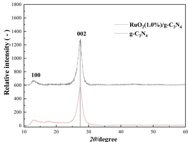
Fig. 2 XRD patterns of bare g-C<sub>3</sub>N<sub>4</sub> and RuO<sub>2</sub> (1.0%)/g-C<sub>3</sub>N<sub>4</sub> composite.
