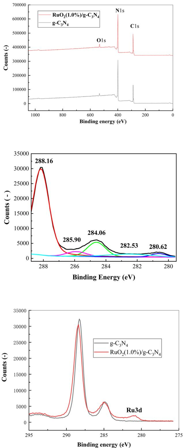
Fig. 5 XPS survey spectra of  $g\text{-C}_3\text{N}_4$  and  $\text{RuO}_2$  (1.0%)/ $g\text{-C}_3\text{N}_4$  (upper), high resolution XPS of  $\text{RuO}_2$  (1.0%)/ $g\text{-C}_3\text{N}_4$  (278–294 eV, middle) and Ru 3d scan of  $\text{RuO}_2$  (1.0%)/ $g\text{-C}_3\text{N}_4$  (lower).
