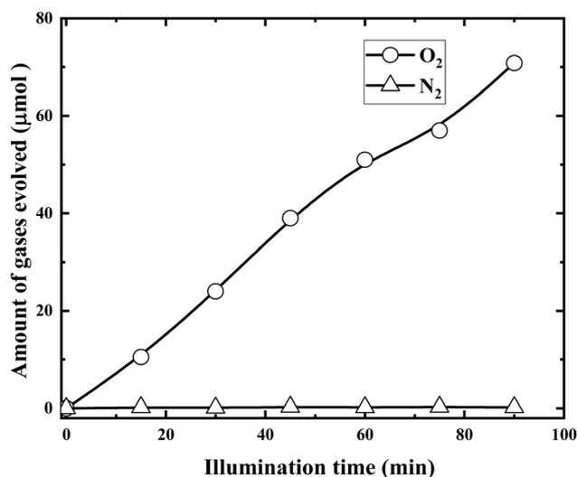
Fig. 15 Time courses of O<sub>2</sub> and N<sub>2</sub> evolution during the illumination (solution volume, 200 mL; RuO<sub>2</sub> (1.0%)/g-C<sub>3</sub>N<sub>4</sub> composite, 0.1 g; initial Cr(vi) concentration, 0.5 mM; pH<sub>0</sub>, 2.4; light source, LED (410 nm, 40 W)).
