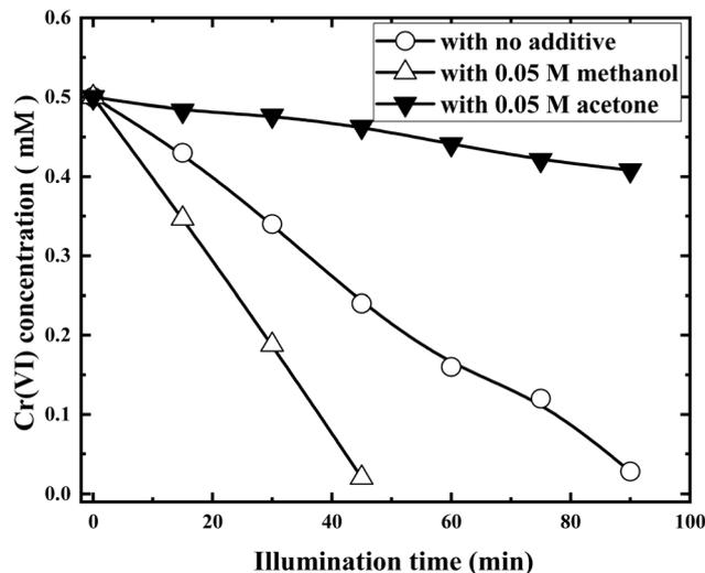
Fig. 10 Photocatalytic reductions of Cr(vi) with RuO<sub>2</sub> (1.0%)/g-C<sub>3</sub>N<sub>4</sub> in the presence of methanol and acetone (solution volume, 200 mL; RuO<sub>2</sub> (1.0%)/g-C<sub>3</sub>N<sub>4</sub> composite, 0.1 g; initial Cr(vi) concentration, 0.5 mM; pH<sub>0</sub>, 2.4; light source, LED (410 nm, 40 W).
