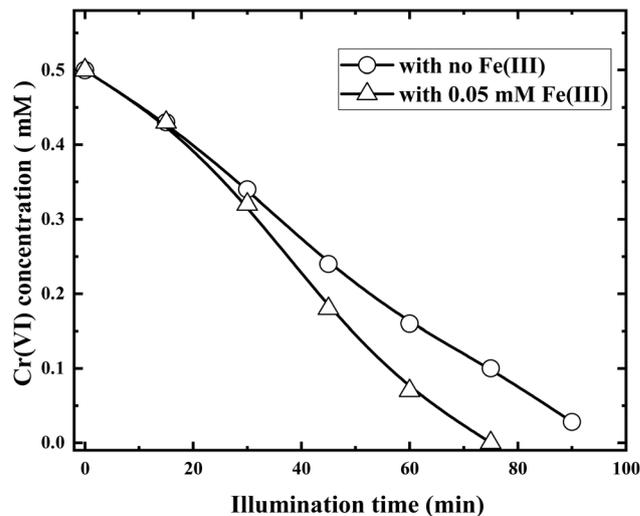
Fig. 11 Photocatalytic reductions of Cr(vi) with RuO<sub>2</sub> (1.0%)/g-C<sub>3</sub>N<sub>4</sub> in the presence and absence of 0.05 mM Fe(III) (solution volume, 200 mL; RuO<sub>2</sub> (1.0%)/g-C<sub>3</sub>N<sub>4</sub> composite, 0.1 g; initial Cr(vi) concentration, 0.5 mM; pH<sub>0</sub>, 2.4; light source, LED (410 nm, 40 W)).
