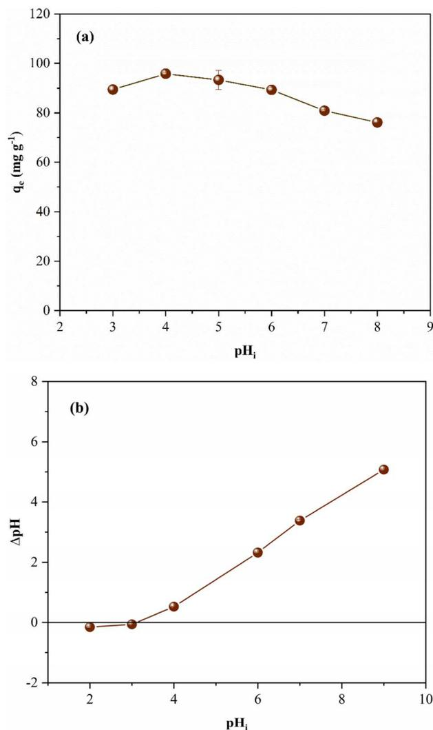
Fig. 7 (a) Effect of solution pH on the TC adsorption capacity, and (b) the  $\text{pH}_{\text{pzc}}$  of M-GO/PFC composite adsorbent.
