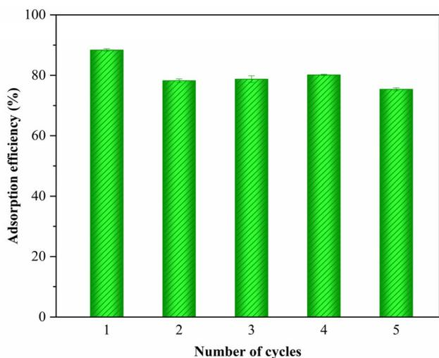
Fig. 12 Recyclability study of M-GO/PFC composite adsorbent.
