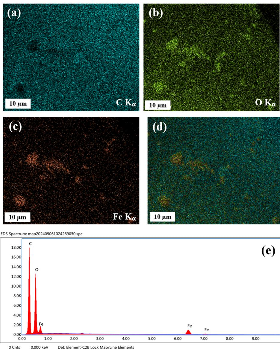
Fig. 5 Elemental maps of (a) C, (b) O, (c) Fe, and (d) M-GO/PFC composite; (e) EDX spectrum of M-GO/PFC composite.
