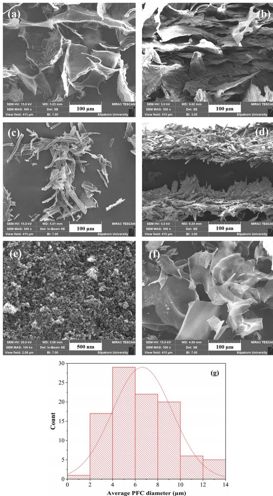
Fig. 4 FE-SEM surface images of (a) GO, (c) PFC, (e) Fe<sub>3</sub>O<sub>4</sub>, and (f) M-GO/PFC composite; FE-SEM cross-section images of (b) GO and (d) PFC; (g) average PFC diameter distribution.
