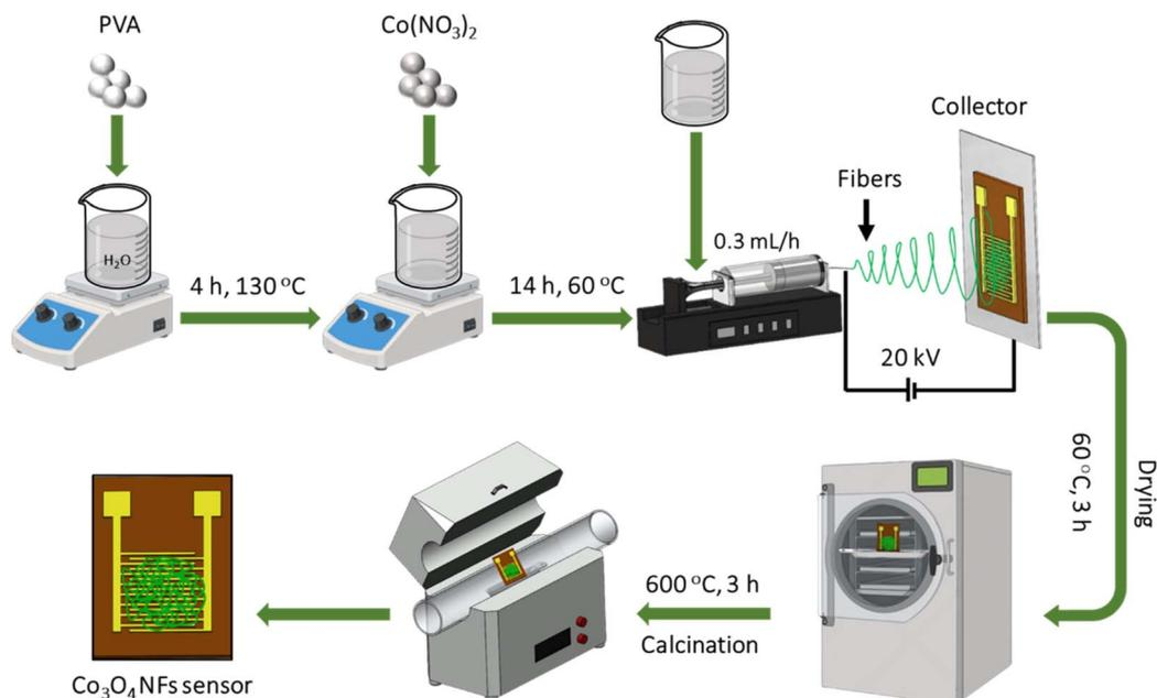
Fig. 1 Synthesis process of  $\text{Co}_3\text{O}_4$  nanofibers sensor.
