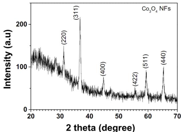
Fig. 6 XRD pattern of the annealed  $\text{Co}_3\text{O}_4$  NFs.
