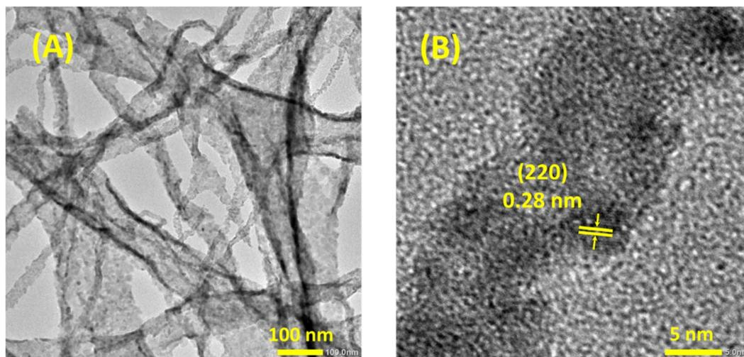
Fig. 7 TEM micrographs featuring the microstructure of annealed  $\text{In}_2\text{O}_3$  polycrystalline nanofibers at varying levels of magnification: (A) lower magnification view and (B) higher magnification view.
