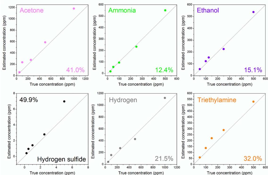
Fig. 10 Estimate of the gas concentration as a function of the true gas concentration for the tested gases.
