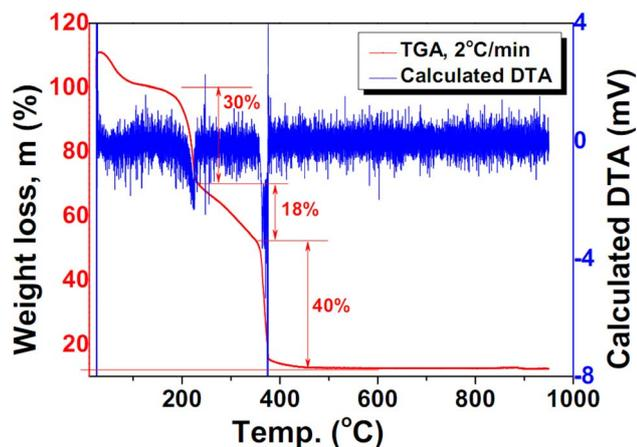
Fig. 4 DTA-TGA curves of the  $\text{Co}(\text{NO}_3)_2/\text{PVA}$  composite nanofibers.
