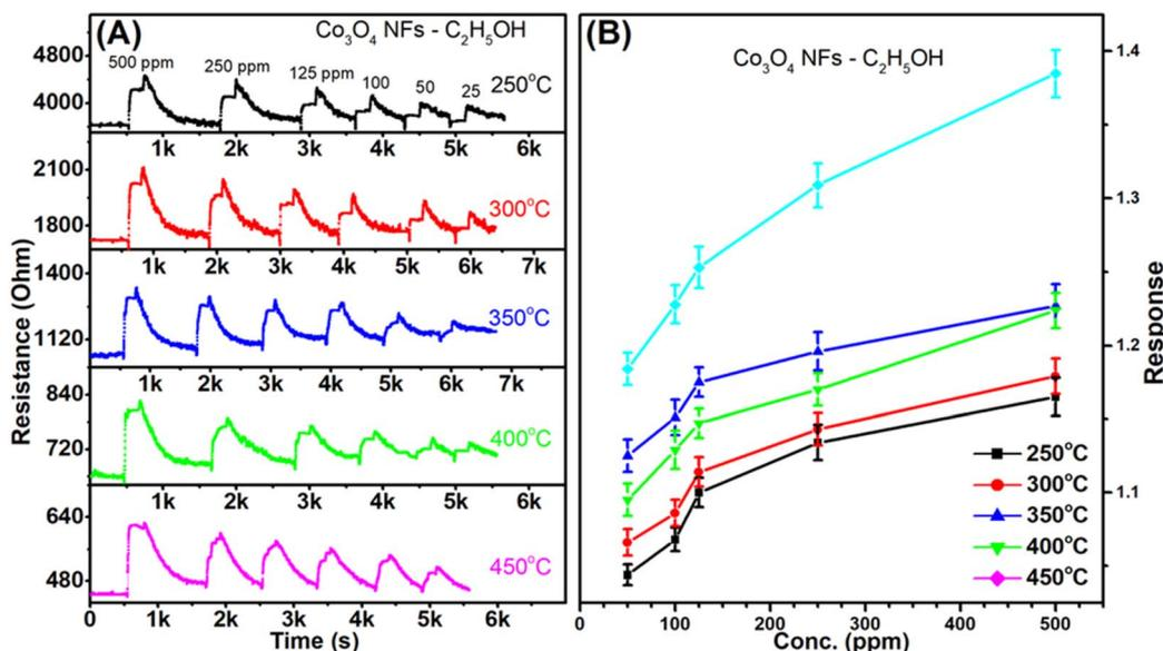
Fig. 8 Ethanol sensing performance of  $\text{Co}_3\text{O}_4$  sensors: (A) dynamic resistance to ethanol concentrations ranging 50–500 ppm at various operating temperatures (250–450 °C); (B) sensor response as a function of ethanol concentration (50–500 ppm) at different working temperatures (250–450 °C).
