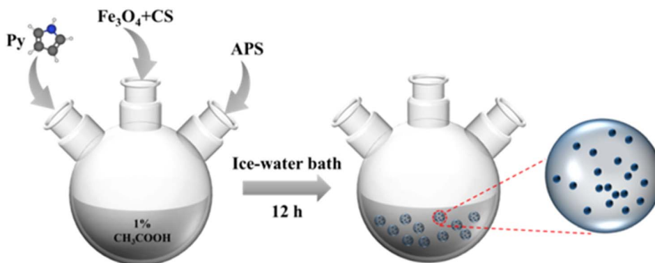
Fig. 1 The synthesis route of the \text{Fe}_3\text{O}_4/\text{CS}/\text{PPy} .
