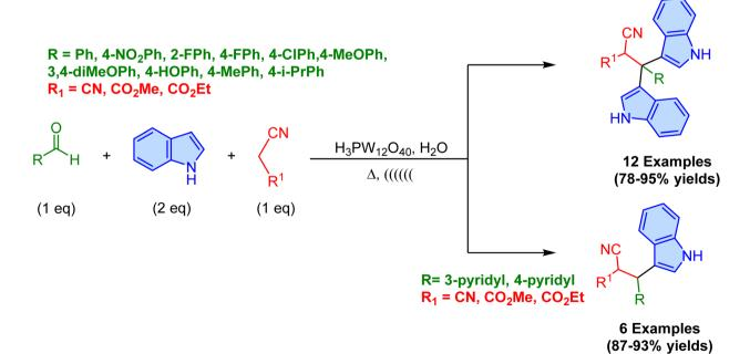
Scheme 34 H<sub>3</sub>PW<sub>12</sub>O<sub>40</sub>-catalyzed solvent-free synthesis of bis(indoles) under silent and ultrasound irradiation.
