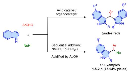
Scheme 7 One-pot sequential synthesis of 3-substituted indoles via NaOH and AcOH catalysis.
