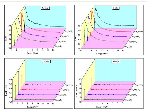
Fig. 12 Graphs between energy absorption build-up factor (EABF) versus photon energy at four different values of penetration depth for all materials in the current study.
