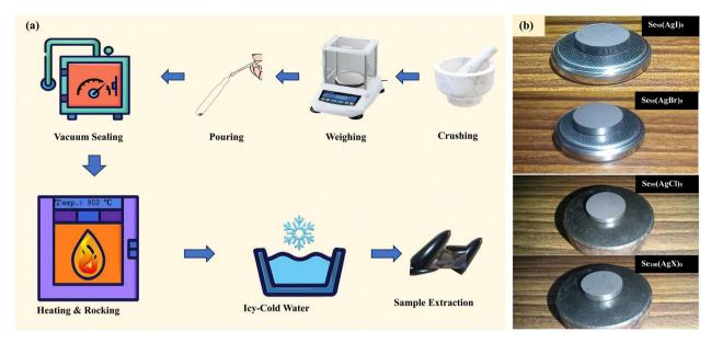
Fig. 1 (a) Synthesis process (b) polished pellet of Se<sub>95</sub>(AgBr)<sub>5</sub> sample.
