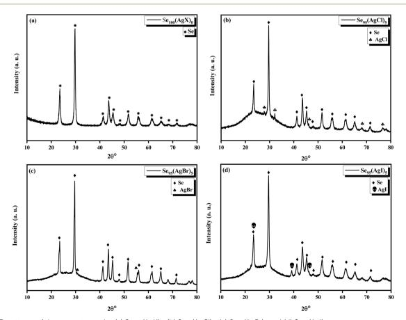
Fig. 2 XRD patterns of the present samples (a)  $Se_{100}(AgX)_0$ , (b)  $Se_{95}(AgCI)_5$ , (c)  $Se_{95}(AgBr)_5$  and (d)  $Se_{95}(AgI)_5$ .
