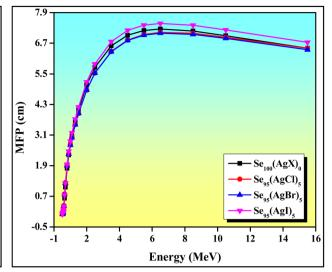
Fig. 7 Variation of half value layer (HVL) and mean free path (MFP) with photon energy for Se and chalcohalide glass ceramics series.
