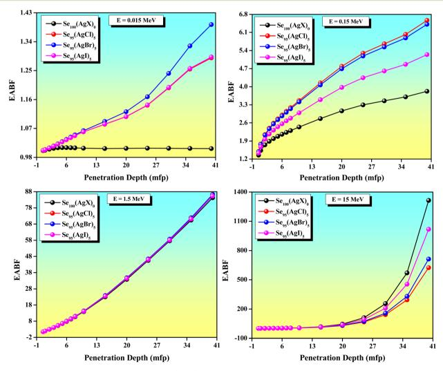
Fig. 10 Variation of energy absorption build-up factor (EABF) with penetration depth at four different values of photon energy for Se and chalcohalide glass-ceramics samples.
