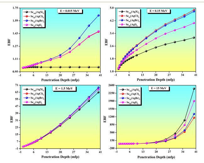
Fig. 11 Variation of exposure build-up factor (EBF) with penetration depth at four different values of photon energy for Se and chalcohalide glass-ceramics samples.
