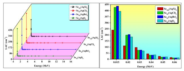
Fig. 6 Dependency of linear attenuation coefficient (LAC) on photon energy for all the samples.
