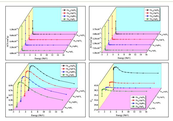
Fig. 9 Graphs between atomic cross-section (ACS), electronic cross-section (ECS), R, and equivalent atomic number ( $Z_{eq}$ ) against photon energy for Se and chalcohalide glass-ceramics.
