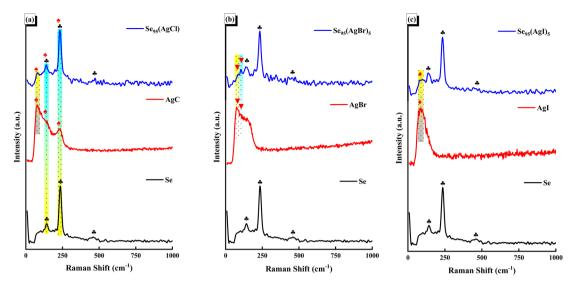
Raman spectra of (a) AgCl, (b) AgBr and (c) AgI-incorporated Se samples at room temperature taken with 532 nm excitation laser.
