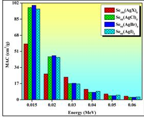
Fig. 5 Dependency of mass attenuation coefficient (MAC) on photon energy for Se and chalcohalide glass ceramics series.
