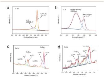
Fig. 2 High-resolution (a) C1s, (b) O1s, (c) Cu2p and (d) Co2p spectra of Cu-Co/BPC.
