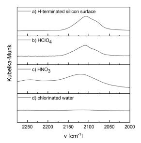
Fig. 1 DRIFT spectra of a (a) H-terminated silicon surface treated with (b) 10.54 mol  $l^{-1}$  HClO<sub>4</sub> for 15 min, (c) 15.44 mol  $l^{-1}$  HNO<sub>3</sub> for 1 min and (d) 0.10 mol  $l^{-1}$  chlorinated water for 1 min. The spectra were measured at a temperature of 20 °C.
