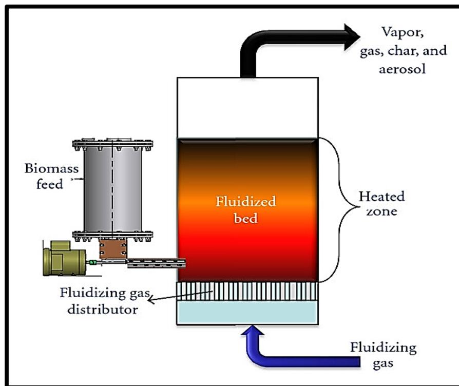
Fig. 17 Schematic of circulating fluidized bed pyrolysis.<sup>155</sup>
