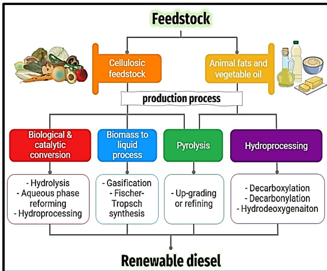
Fig. 18 Catalytic processing for biomass conversion towards fuels production.<sup>19</sup>
