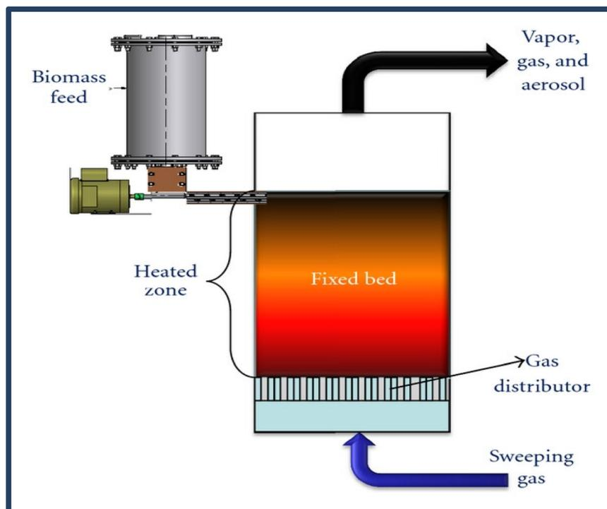
Fig. 15 Fixed bed reactor for biomass pyrolysis<sup>155</sup>
