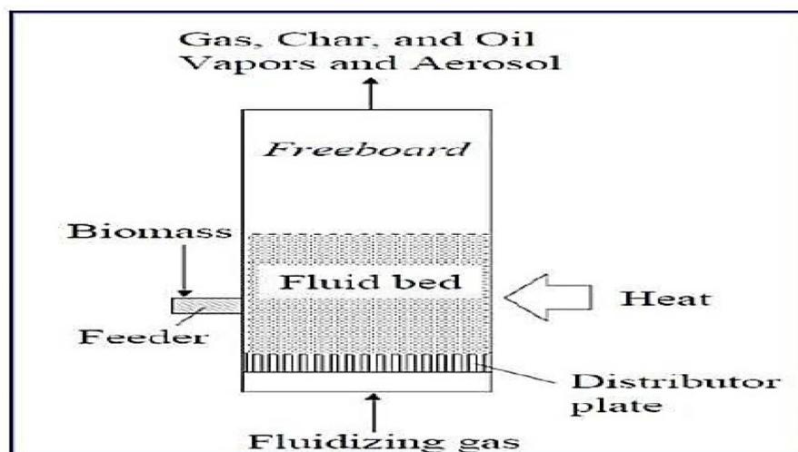
Fig. 16 Bubbling fluidized-bed reactor.<sup>157</sup>
