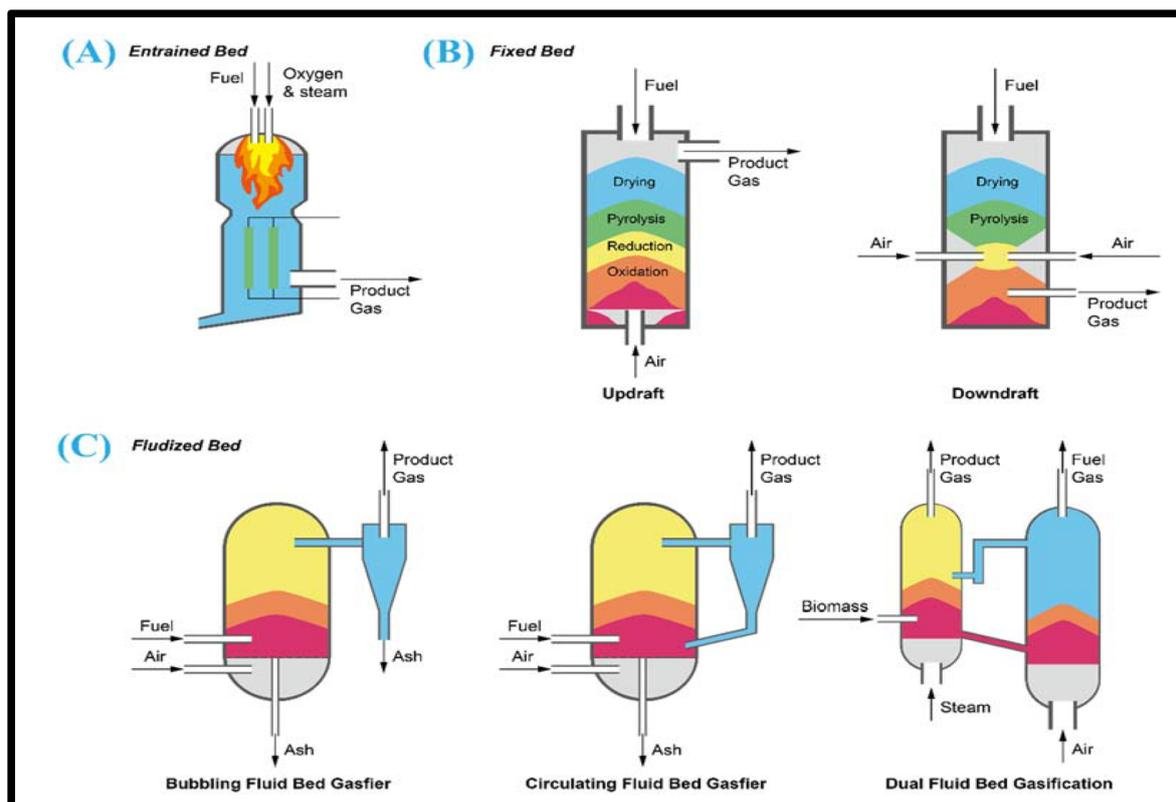
Fig. 13 Types of gasifiers (A) entrained bed, (B) fixed bed, and (C) fluidized bed.<sup>142</sup>
