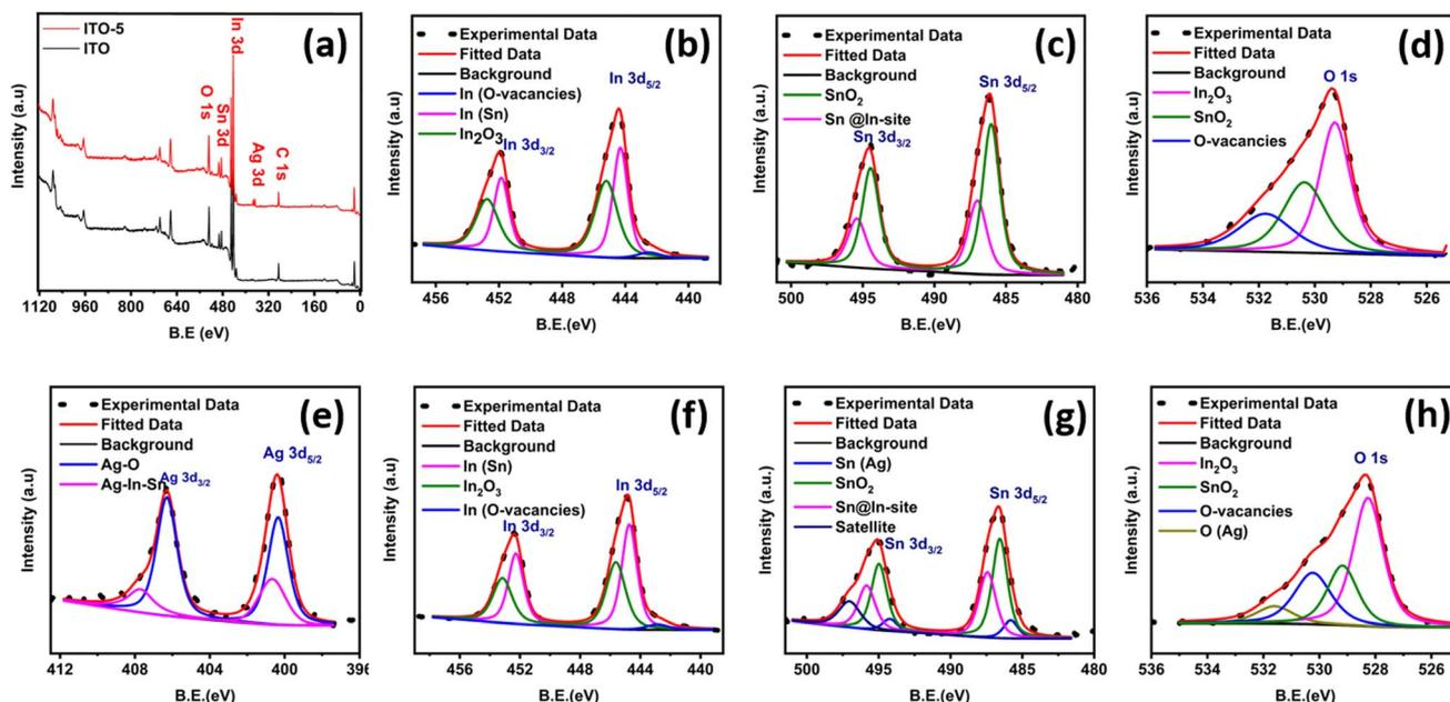
Fig. 2 XPS analysis, a full survey scans of ITO and ITO-5 (a). High-resolution spectra of In, Sn and O from ITO (b–d). High-resolution spectra of In, Sn, O and Ag from ITO-5 (e–h).
