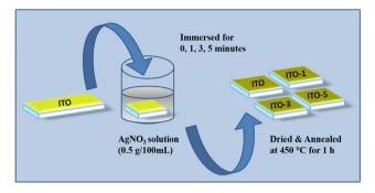
Fig. 1 Schematic representation of silver incorporated on ITO films.
