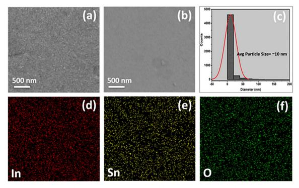
Fig. 3 SEM micrographs of pure ITO (a) secondary electron (SE) image (b) backscattered electron (BSE) image (c) particle size distribution estimated by ImageJ software (d-f) elemental distribution of indium (In), tin (Sn) and oxygen (O) images by energy dispersive spectroscopy (EDS).
