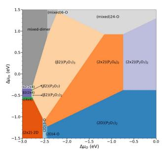
Fig. 6 Overall phase diagram of the oxygenated InP(001) surface, showing the most stable surface reconstructions as function of the chemical potentials of indium and oxygen.
