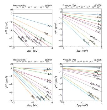
Fig. 4 Surface energy wrt. oxygen chemical potential of the energetically favourable O adsorption sites for (a)  $(2 \times 2)$ , (b)  $(2 \times 2)$ -2D, (c) mixed-dimer and (d)  $\beta 2(2 \times 4)$  surface reconstructions.
