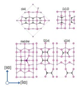
Fig. 2 Ball-and-stick representation for stable InP(001) surface reconstructions, viewed along the (001) surface normal. Surface dimers, i.e. P-dimers are indicated in dark grey, and In-P dimers are indicated in a magenta-dark grey format. In and P atoms are indicated by pink and grey respectively.
