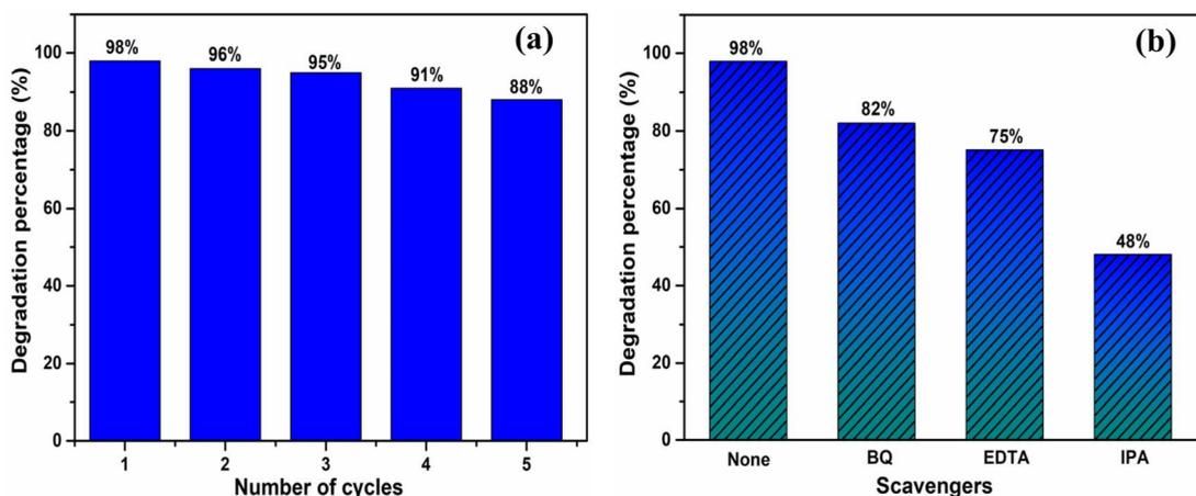
Fig. 6 (a) Recycling performance and (b) trapping experiment for photocatalytic degradation of MB solution over  $\text{TiO}_2@rGO-hBN$  under UV light irradiation.
