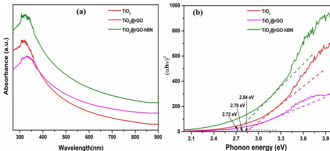
Fig. 3 (a) UV-vis absorption spectra and (b) optical band gap of  $\text{TiO}_2$ ,  $\text{TiO}_2$ @rGO and  $\text{TiO}_2$ @rGO-hBN.
