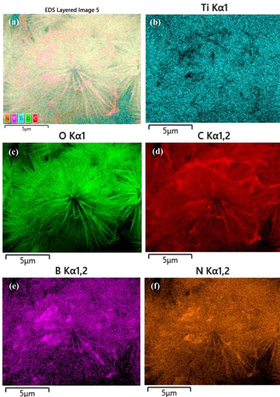
Fig. 2 (a) SEM mapping image and elemental mapping images of (b) Ti, (c) O, (d) C, (e) B and (f) N elements of  $\text{TiO}_2@r\text{GO-hBN}$ .
