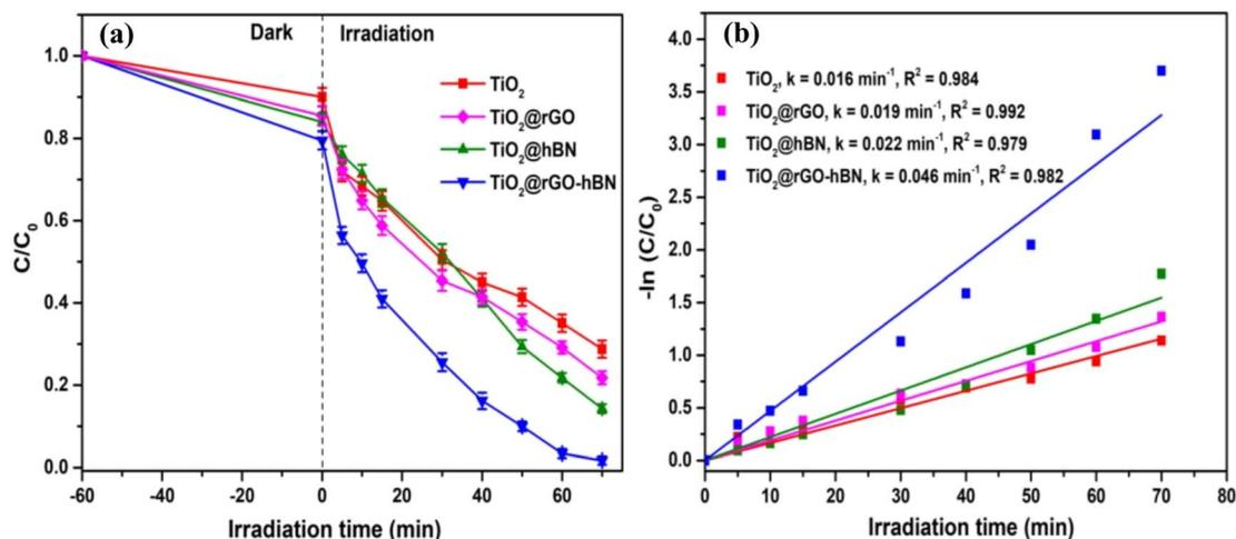
Fig. 5 Comparison of (a) photocatalytic activity and (b) apparent rate constants ( $k$ ) of  $\text{TiO}_2$ ,  $\text{TiO}_2@rGO$ ,  $\text{TiO}_2@hBN$  and  $\text{TiO}_2@rGO-hBN$  towards photocatalytic degradation of MB solution under UV light irradiation.
