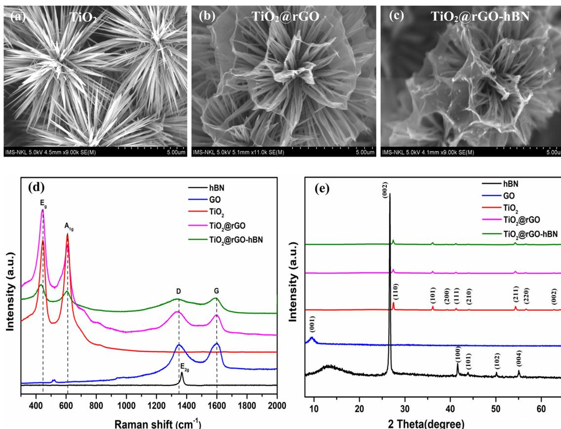
Fig. 1 SEM images of (a)  $\text{TiO}_2$ , (b)  $\text{TiO}_2$ @rGO and (c)  $\text{TiO}_2$ @rGO-hBN. Raman spectra (d) and XRD pattern (e) of hBN, GO,  $\text{TiO}_2$ ,  $\text{TiO}_2$ @rGO and  $\text{TiO}_2$ @rGO-hBN.
