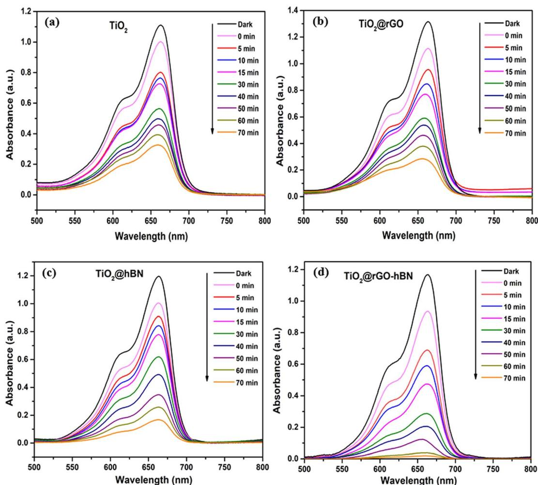
Fig. 4 Photodegradation absorption spectra of MB solution in (a)  $\text{TiO}_2$ , (b)  $\text{TiO}_2$ @rGO, (c)  $\text{TiO}_2$ @hBN and (d)  $\text{TiO}_2$ @rGO-hBN.
